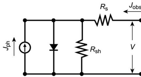
Fig. 4 Equivalent circuit of OPV devices.
