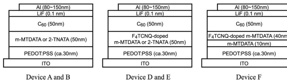
**Fig. 1** Structures of fabricated devices.
