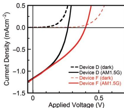
**Fig. 5**  $J$ - $V$  characteristics of device D and device F in the dark and under AM1.5G illumination at an incident light intensity of  $100 \text{ mW cm}^{-2}$ .
