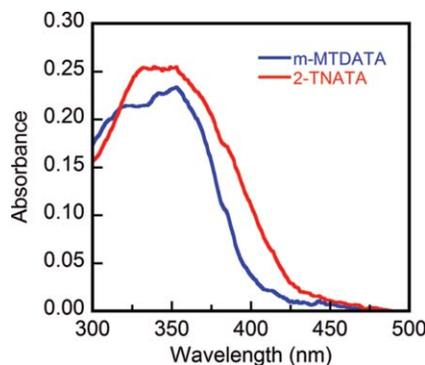
**Fig. 3** Electronic absorption spectra of vapor-deposited films of m-MTDATA (30 nm) and 2-TNATA (30 nm).
