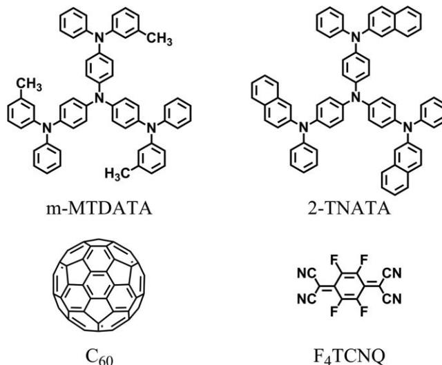
In the present study, we have investigated the effect of *p*-type doping of the donor layer with F<sub>4</sub>TCNQ on the performance of planar *pn*-heterojunction OPV devices. Amorphous molecular materials with low solid state ionization potentials ( $I_p$ s), m-MTDATA ( $I_p$  5.1 eV,<sup>49</sup>) and
