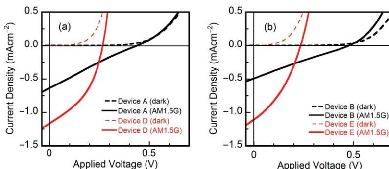
**Fig. 2** *J*–*V* characteristics of (a) device A and device D, and (b) device B and device E in the dark and under AM1.5G illumination at an incident light intensity of 100 mW cm<sup>-2</sup>.
