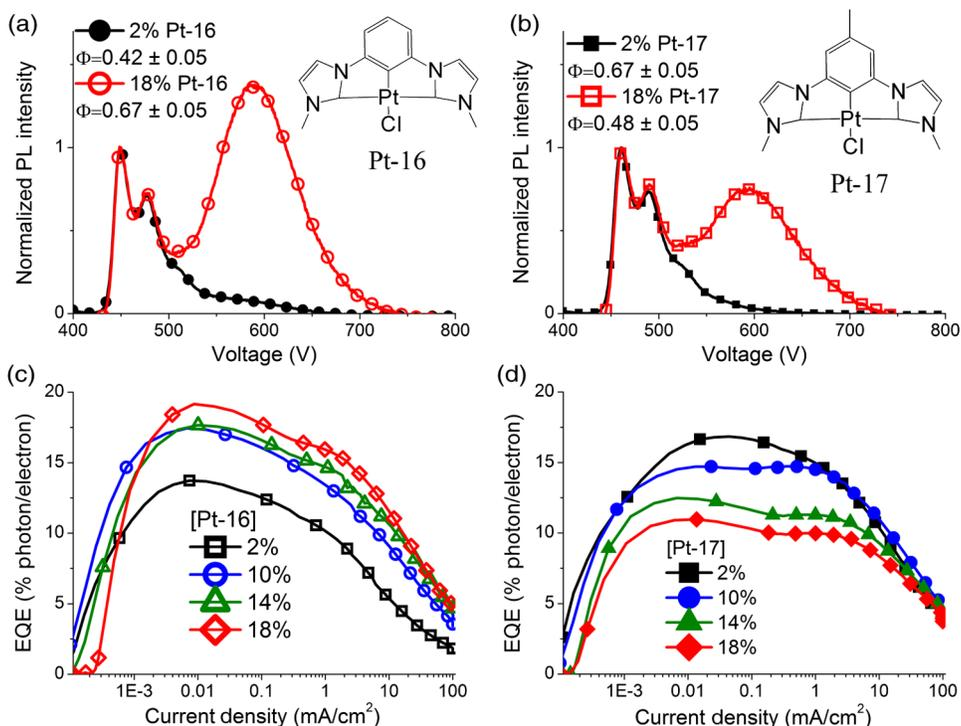
**Fig. 4** Thin film photoluminescent (PL) spectra for (a) Pt-16 and (b) Pt-17 for 2% and 18% dopant concentrations with the respective quantum yields inset in the figure and the external quantum efficiency (EQE) as a function of concentration for (c) Pt-16 and (d) Pt-17 for devices in the structure: ITO/PEDOT:PSS/NPD (30 nm)/TAPC (10 nm)/x% emitter:26mCPy (25 nm)/PO15 (40 nm)/LiF/Al. Data from Ref 35.
