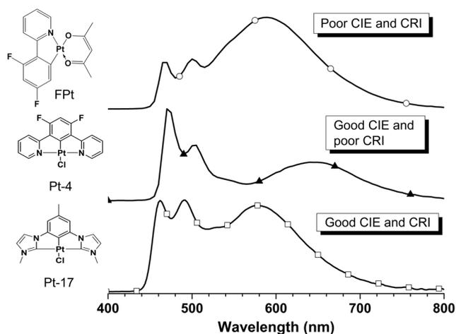
**Fig. 3** Electroluminescent spectra of devices using FPt, Pt-4, and Pt-17 with their corresponding chemical structures on the left (from Ref. 54).
