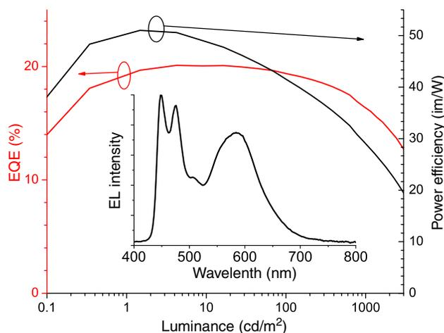
**Fig. 8** EQE and power efficiency (PE) versus luminance and electroluminescent (EL) spectrum of a WOLED in the structure: ITO/PEDOT:PSS (20 nm)/TAPC (25 nm)/10% **25** in TAPC:PO15 (1:1) (10 nm)/PO15 (30 nm)/BmPyPB/LiF/Al.
