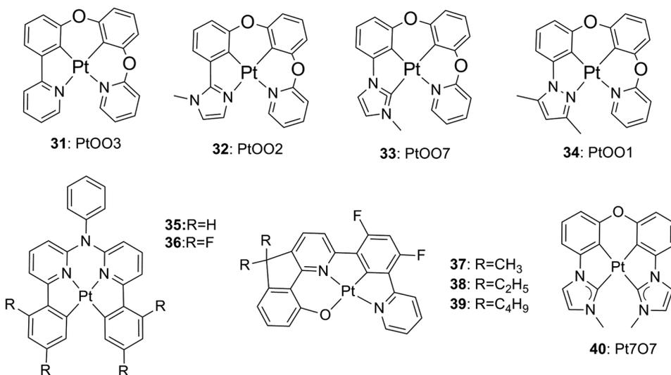
**Fig. 9** Selected tetradentate Pt complexes used for excimer emitting WOLEDs.
