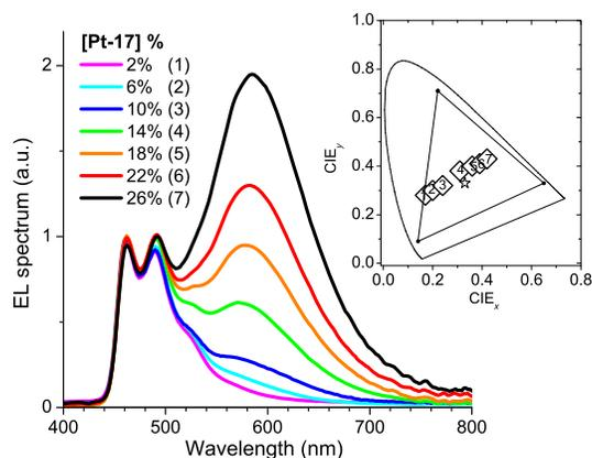
**Fig. 2** Color variation as a function of dopant concentration for an excimer-based white device in the structure: ITO/PEDOT/NPD (30 nm)/TAPC (10 nm)/x% Pt-17:26 mCpY (25 nm)/PO15 (20 nm)/LiF/Al (from Ref. 54).
