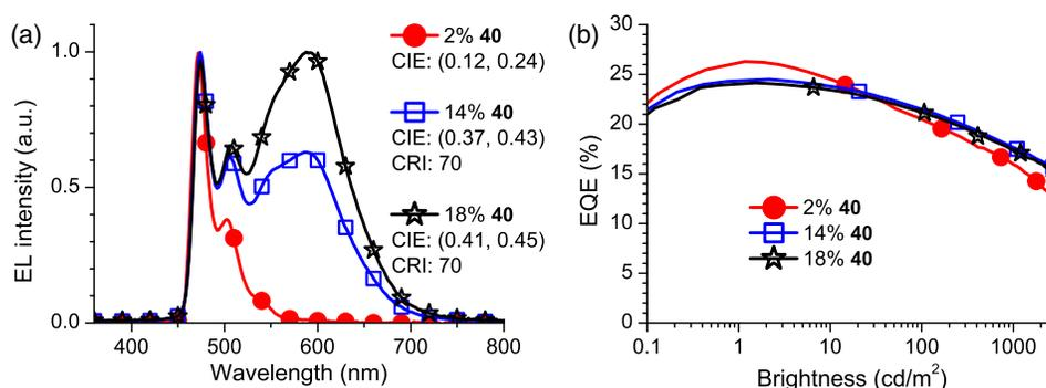
**Fig. 10** (a) EL spectra and (b) EQE versus brightness for devices of complex **40** as a function of concentration in the structure: ITO/HATCN (10 nm)/NPD (40 nm)/TAPC (10 nm)/*x*% **40**:mCBP (25 nm)/DPPS (10 nm)/BmPyPB (40 nm)/LiF/Al.
