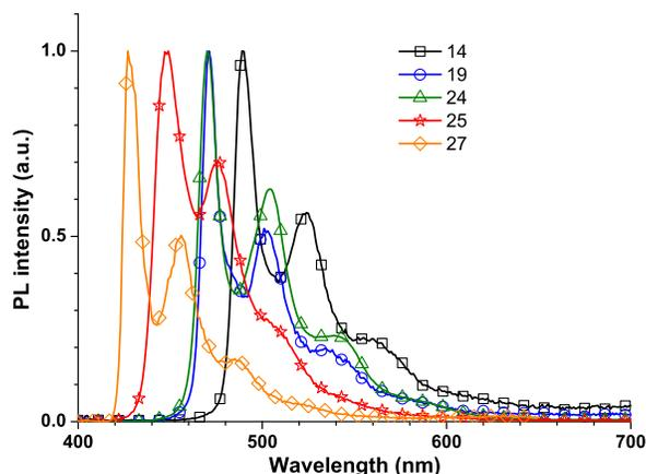
**Fig. 7** The PL emission spectra of **14**, **19**, **24**, and **25** in a solution of  $\text{CH}_2\text{Cl}_2$  at room temperature and of **27** in a 2% PMMA thin film.
