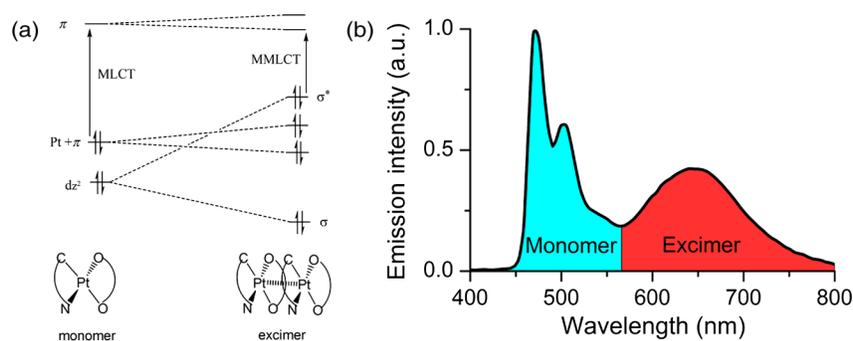
**Fig. 1** (a) Example of formation of phosphorescent excimer and (b) example of a typical emission spectrum observed for excimer based WOLEDs.
