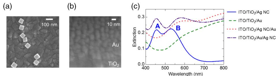
**Fig. 1** Scanning electron micrographs of (a) the Ag NCs and (b) the Au films. (c) Extinction spectra of the ITO/TiO<sub>2</sub>/Ag NC, ITO/TiO<sub>2</sub>/Ag NC/Au, ITO/TiO<sub>2</sub>/Au, and ITO/TiO<sub>2</sub>/Au/Ag NC electrodes in water.
