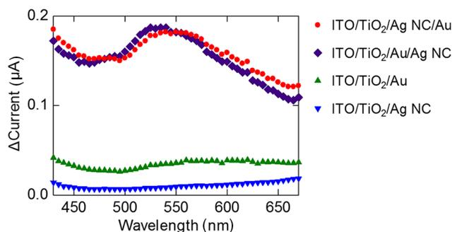
**Fig. 2** Photocurrent action spectra of the ITO/ $\text{TiO}_2$ /Ag NC, ITO/ $\text{TiO}_2$ /Ag NC/Au, ITO/ $\text{TiO}_2$ /Au, and ITO/ $\text{TiO}_2$ /Au/Ag NC electrodes in 0.1-M aqueous  $\text{KNO}_3$  containing 0.5-M ethanol. Each datapoint shows the average of photocurrent responses from three independently prepared electrodes.
