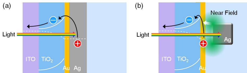
**Fig. 4** Possible mechanisms of (a) the PICS with accelerated electron transfer and (b) PICS enhanced by the nanoantenna effect.
