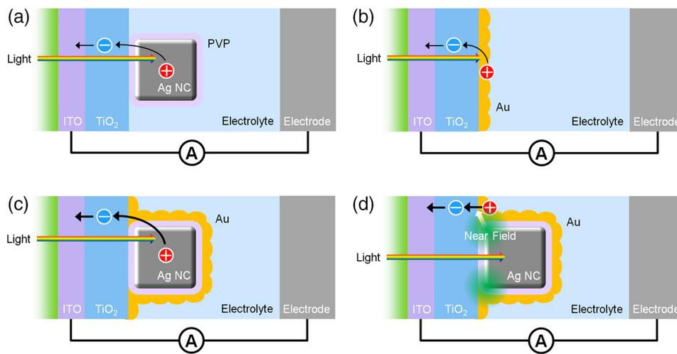
**Fig. 3** Possible mechanisms of the photocurrents based on PICS for (a) ITO/ $\text{TiO}_2$ /Ag NC, (b) ITO/ $\text{TiO}_2$ /Au, and (c and d) ITO/ $\text{TiO}_2$ /Ag NC/Au electrodes [(c) PICS with accelerated electron transfer and (d) PICS enhanced by the nanoantenna effect].
