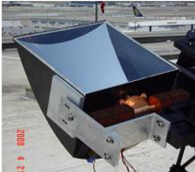
Fig. 8. Prototype B module under test at the Boeing Solar test site in El Segundo, CA.
