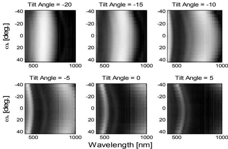
Figure 2: Measured diffraction efficiency as a function of reconstruction and tilt angles with different reconstruction wavelengths.
