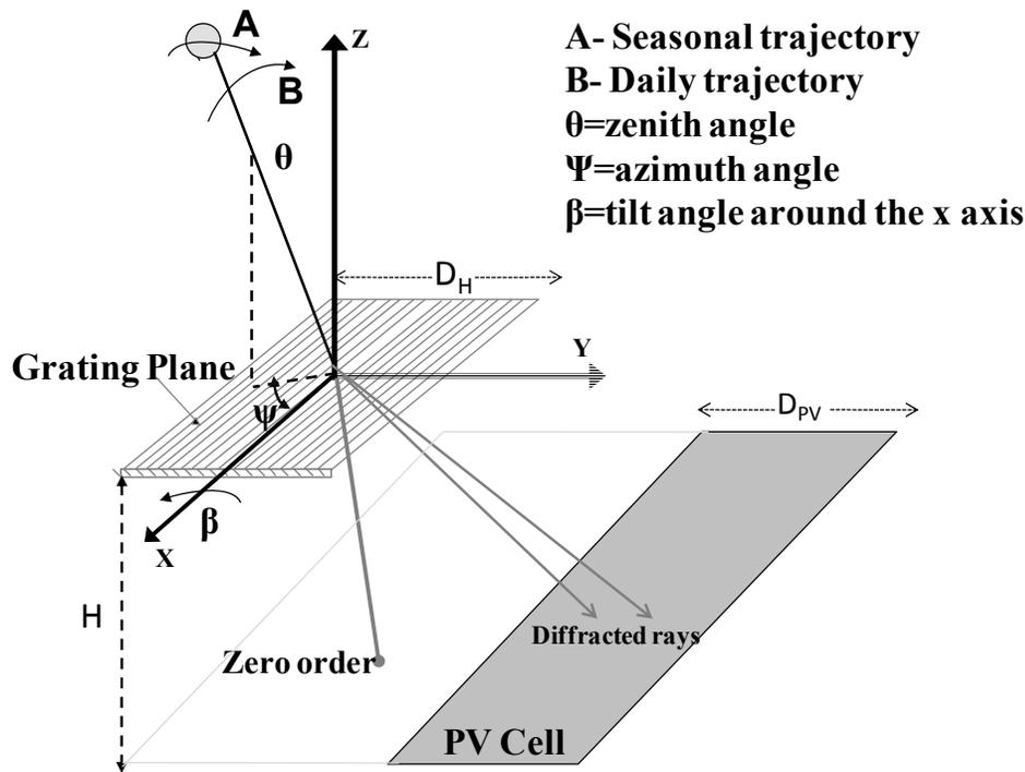
Figure 4: Geometry used for the holographic planar concentrator.
