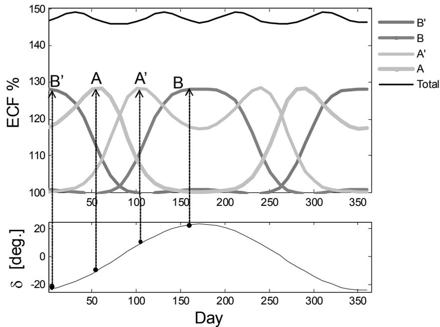
Figure 7: ECE obtained with two cascaded holograms (A,B) on the left side of the PV cell and (A',B') on the right side of the cell.
