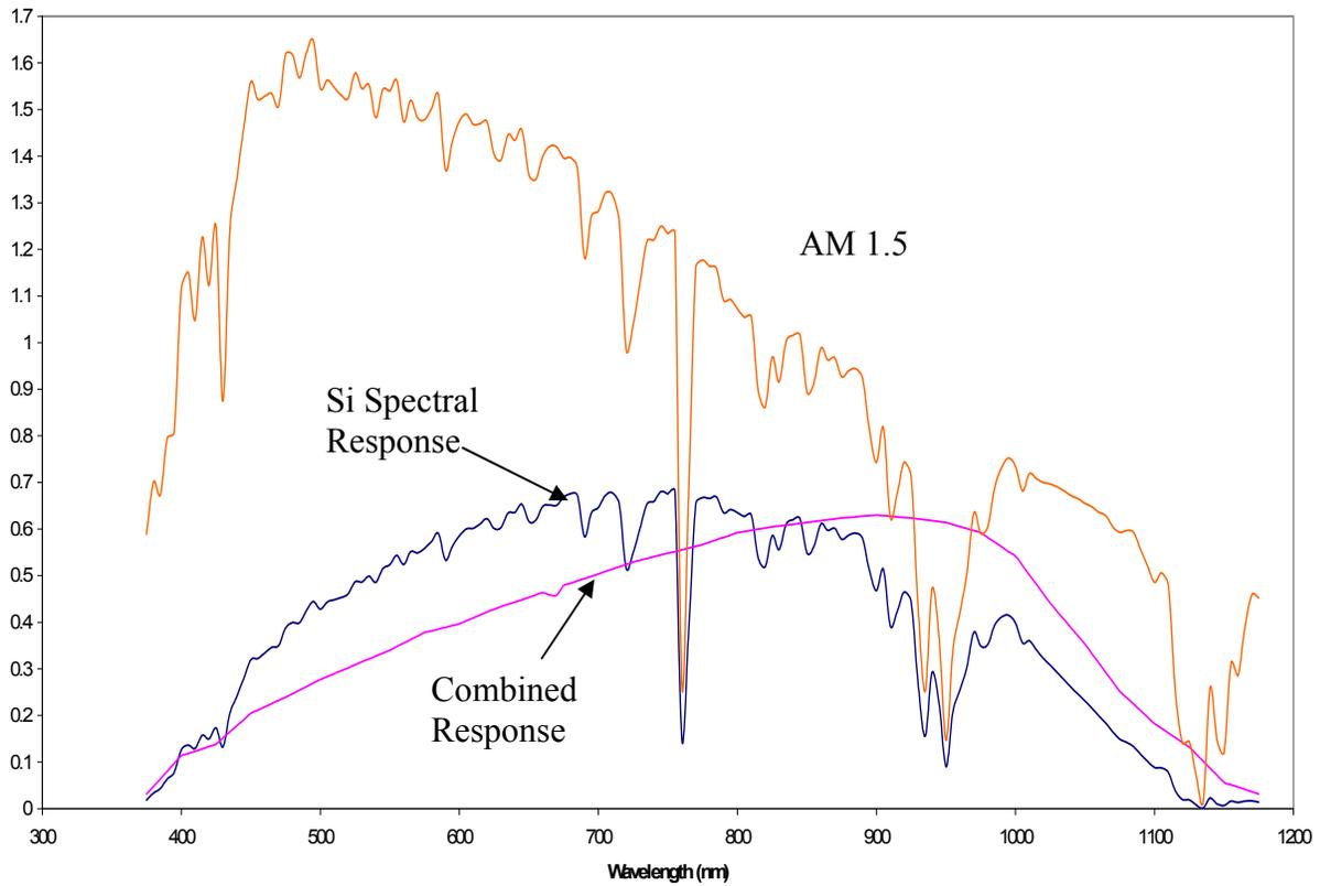
Figure 5: Spectral irradiance corresponding to solar illumination with and air mass of 1.5, the spectral responsivity of a silicon PV cell, and a combined spectral response.
