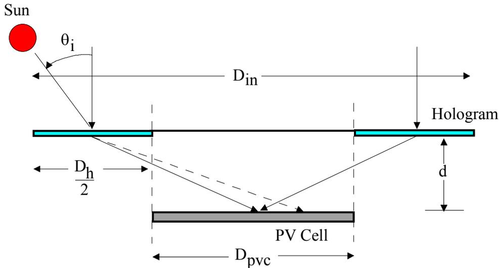
Figure 3: Schematic diagram for a holographic planar concentrator with the hologram area ( $D_h$ ) split on each side of the PV cell area ( $D_{pvc}$ )
