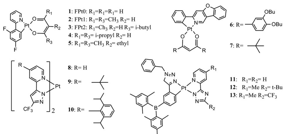
**Fig. 5** Selected bidentate Pt complexes used for excimer emitting white organic light emitting diodes (WOLEDs).
