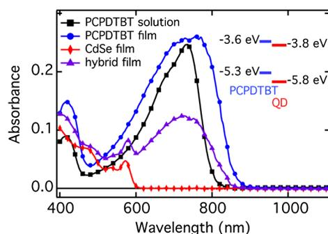
**Fig. 1** Representative steady-state absorption spectra of the donor and acceptor components of the BHJs studied: PCPDTBT solution (square), PCPDTBT film (circles), CdSe nanocrystal film (diamonds), and hybrid BHJ film composed of PCPDTBT:CdSe nanocrystals (triangles). The inset shows the frontier energy levels of the PCPDTBT polymer and of the CdSe nanocrystals, which were determined by electrochemistry for each individual component.<sup>19</sup>
