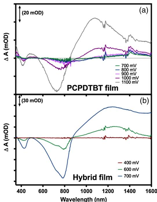
**Fig. 5** Difference steady state absorption spectra obtained from spectroelectrochemical measurements on (a) neat PCPDTBT films and (b) hybrid PCPDTBT:CdSe BJJ films. The films were spun-cast onto ITO substrates, which acted as the working electrode. A Pt-wire counter electrode and Ag-wire pseudoreference electrode were used to complete the three-electrode setup. Measurements were performed in an acetonitrile solution of 0.1 M tetrabutylammonium hexafluorophosphate.
