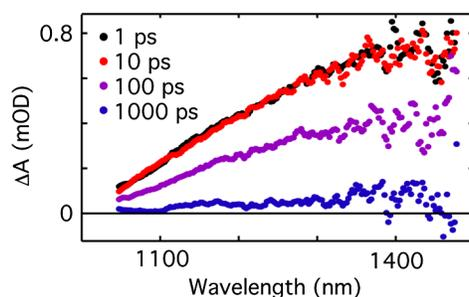
**Fig. 2** Transient absorption (TA) spectra of a PCPDTBT solution for various delays between the pump and the probe pulses.  $\lambda_{\text{exc}} = 800 \text{ nm}$ , pump fluence =  $200 \mu\text{J cm}^{-2}$ .
