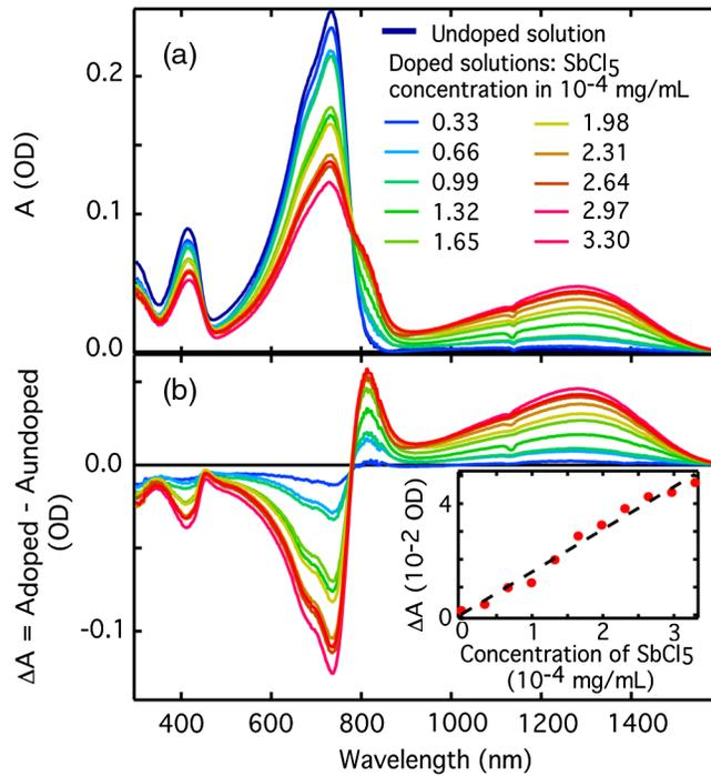
**Fig. 3** (a) PCPDTBT solution steady-state absorption spectra for different  $\text{SbCl}_5$  dopant concentrations using a fixed polymer concentration of  $33 \mu\text{g mL}^{-1}$  in DCB. (b) Difference spectra for the raw absorbance data shown in (a). The inset of (b) details the determination of the polaron absorption coefficient at 1284 nm. Measurements were taken in an integrating sphere and therefore account for scattering and reflections.
