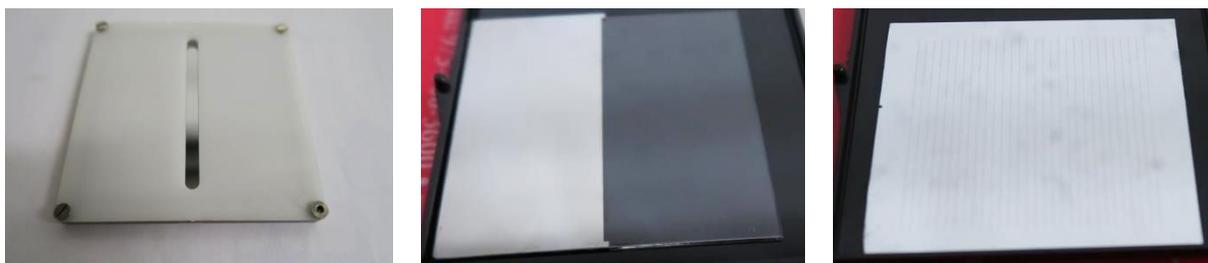
Fig. 6. Different objects that will be placed at the entrance of CSL Offner relay. (Left) 7.5µm wide slit for alignment and MTF. (Center) Knife-edge for the straylight measurement. (Right) Array of 50µm wide slits for keystone measurement.
