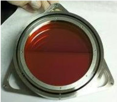
Finally comparing the two different approaches to obtain the desired flatness of the optic we can consider that while Case\_1 (SiO<sub>2</sub> Compensantion) is definitely easier to control and apply for quartz substrates, Case\_2 can be applied to any substrate material.
