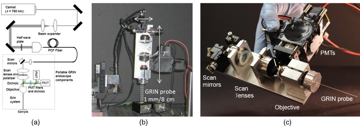
**Fig. 1** Portable GRIN endoscope. (a) Optical drawing and (b) photograph of the GRIN-based endoscope system as mounted for imaging and (c) close up of the portable GRIN endoscope.
