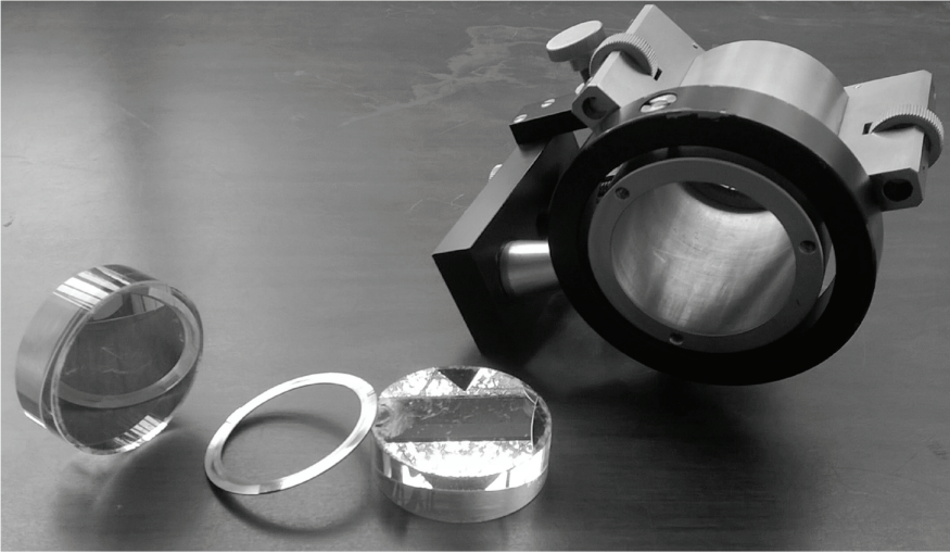
Figure 3.58 A basic Fabry-Pérot interferometer. It consists of two flat mirrors of semi-silvered glass on one of the faces, a spacer ring ( \sim 0.5 mm thick), and a cylindrical support that adjusts the mirror system with the spacer in the middle.
