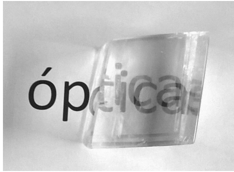
Figure 2.27 Double image generated with a calcite crystal.
