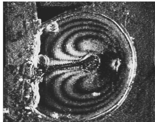
**Fig. 8** Moiré interferogram obtained with our apparatus on the same membrane as in Figure 6, but now with the difference taken between the grid line image on the membrane in its resting position and the grid line image on the membrane deformed by a static pressure of  $2 \text{ kPa}$ . The fringes now represent contours of equal displacement, again with a step of  $0.082 \text{ mm}$  per fringe order.
