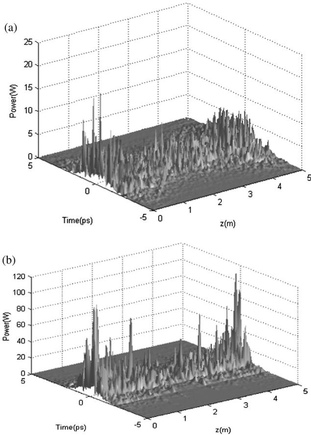
**Fig. 3** Evolution of substructure in a 5 m ring resonator when pulses grow from spontaneous emission with group-velocity dispersion: (a)  $\beta_2 = -0.014 \text{ ps}^2/\text{m}$ , (b)  $\beta_2 = -0.012 \text{ ps}^2/\text{m}$ . Other parameters are  $\gamma = 0.012 \text{ (Wm)}^{-1}$ ,  $\alpha_2 = 0.3$ ,  $T_2 = 0.047 \text{ ps}$ ,  $\alpha = 0.17823 \text{ m}^{-1}$ , and  $g = 0.78275 \text{ m}^{-1}$ .
