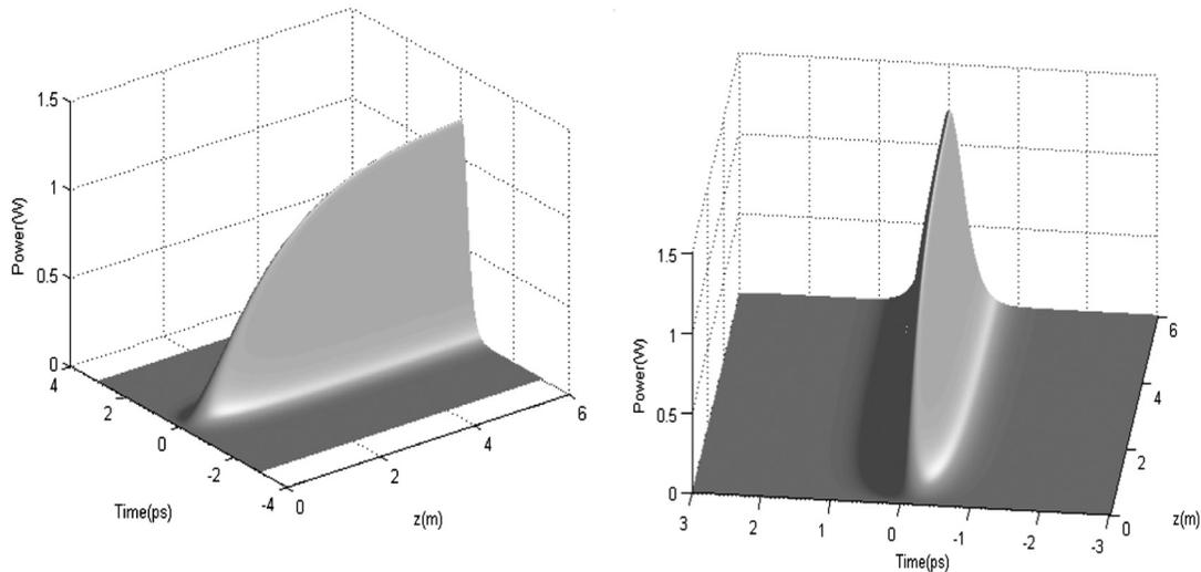
**Fig. 4** Soliton growth from spontaneous emission with erbium-doped fiber laser parameters of  $\gamma = 0.012 \text{ (Wm)}^{-1}$ ,  $\beta_2 = -0.012 \text{ ps}^2/\text{m}$ ,  $\alpha_2 = 0.3$ ,  $T_2 = 0.047 \text{ ps}$ ,  $\alpha = 0.17823 \text{ m}^{-1}$ ,  $g = 0.78275 \text{ m}^{-1}$ ,  $\delta_{\text{SA}} = 0.1$  and  $p_{\text{sat}} = 210 \text{ W}$ .
