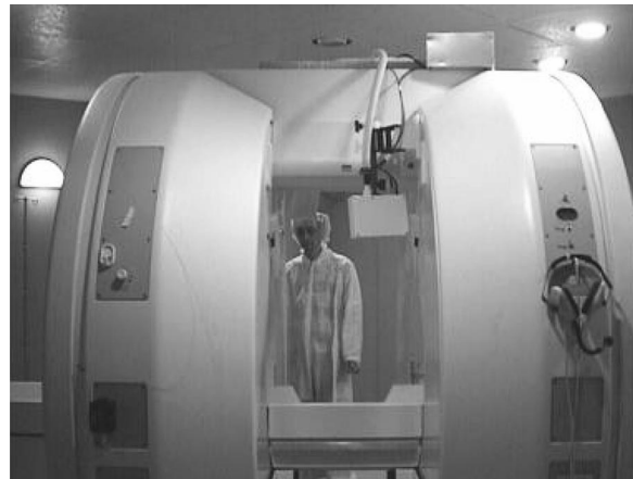
Fig. 2 The open-configuration interventional MRI unit with 0.5 T superconducting magnets and 56 cm gap for surgical access provides a spherical imaging volume 30 cm in diameter. The scan plane can be determined by keyboard at a conventional console, or interactively determined by detection/localization system.
