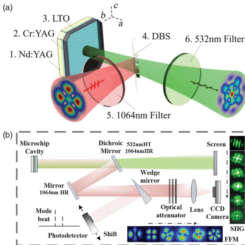
**Fig. 6** Diagram of (a) the experimental principle and (b) setup of the SHG process of TML beams. In panel (a), 1: Nd:YAG microchip; 2: Cr:YAG microchip; 3: LTO, LiTaO<sub>3</sub> microchip; 4: DBS, dichroic beam splitter; 5: 532 nm filter; 6: 1064 nm filter; and  $a$ ,  $b$ ,  $c$  represent the crystallographic axes;  $c$  is also the optical axis. (b) The experimental setup and some beam patterns of both the fundamental frequency and SHG beams.
