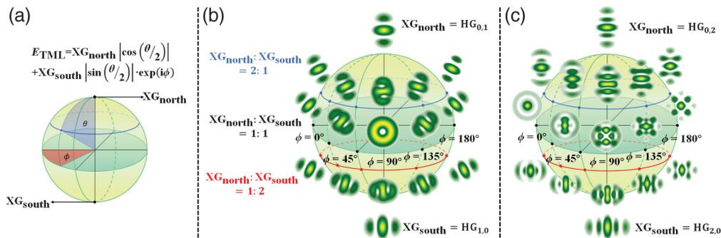
**Fig. 3** Far-field SHG beam patterns of various TML beams marked on the Poincaré sphere. (a) The point  $(\theta, \phi)$  on the Poincaré sphere represents a particular TML state of  $E_{\text{TML}} = XG_{\text{north}} \left| \cos(\theta/2) \right| + XG_{\text{south}} \left| \sin(\theta/2) \right| \cdot \exp(i\phi)$ . (b) and (c) The corresponding far-field SHG beam patterns of different TML states with  $HG_{0,1} \oplus HG_{1,0}$  and  $HG_{0,2} \oplus HG_{2,0}$ , respectively.
