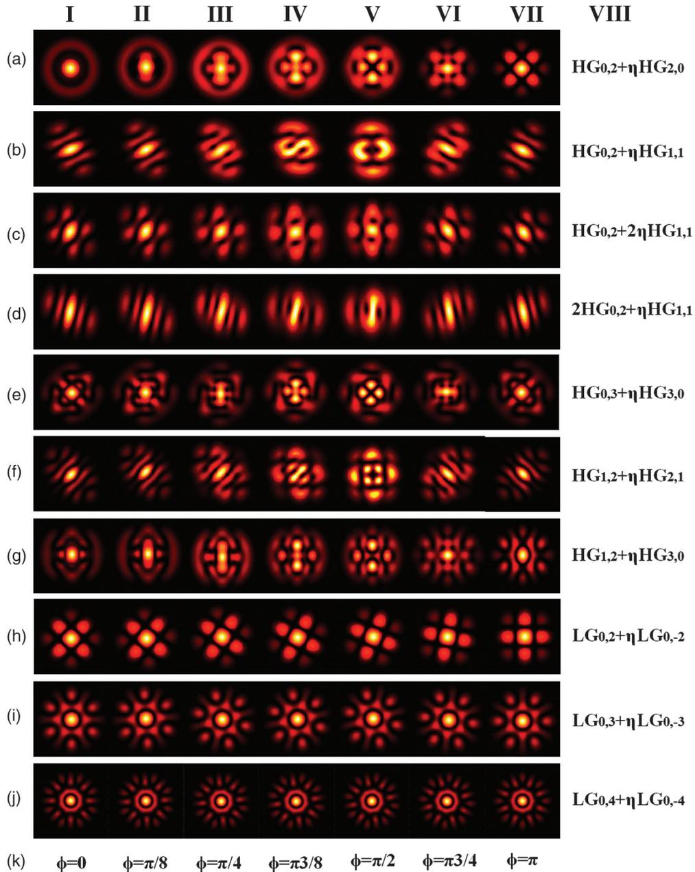
**Fig. 4** Simulated far-field beam patterns of SHG beams corresponding to different TML beams. In column VIII, the TML beams' equations based on Eq. (1) are given. In rows (a) to (g) and rows (h) to (j), different far-field patterns of SHG beams of transverse mode locking states with two HG and LG modes are given, respectively. Here,  $\eta = \exp(i\phi)$ . In row (k), the exact values of the locking phase difference  $\phi$  are given.
