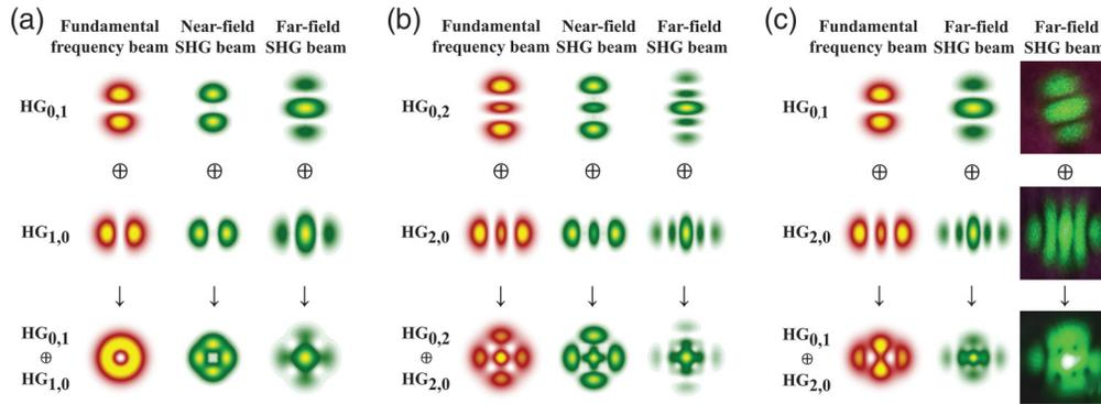
**Fig. 2** The mode compositions in (a), (b), and (c) are  $HG_{0,1} \oplus HG_{1,0}$ ,  $HG_{0,2} \oplus HG_{2,0}$ , and  $HG_{0,1} \oplus HG_{2,0}$ . Here,  $\oplus$  represents the incoherent superposition of the modes. The first and second rows are far-field patterns of two basic HG modes and the third row is the direct intensity superposition of the above two rows.
