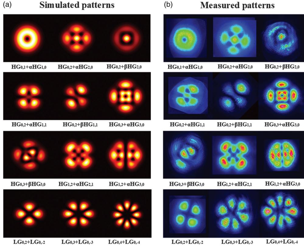
**Fig. 1** Several examples of the fundamental frequency beam patterns in TML states to show the possibility of the generation of TML beams by a microchip cavity. (a) Simulations of the far-field beam pattern of TML modes; (b) corresponding experimental results of the far-field beam patterns of TML modes. Here,  $\alpha = \exp(i\pi/2)$  and  $\beta = \exp(i\pi/4)$ .
