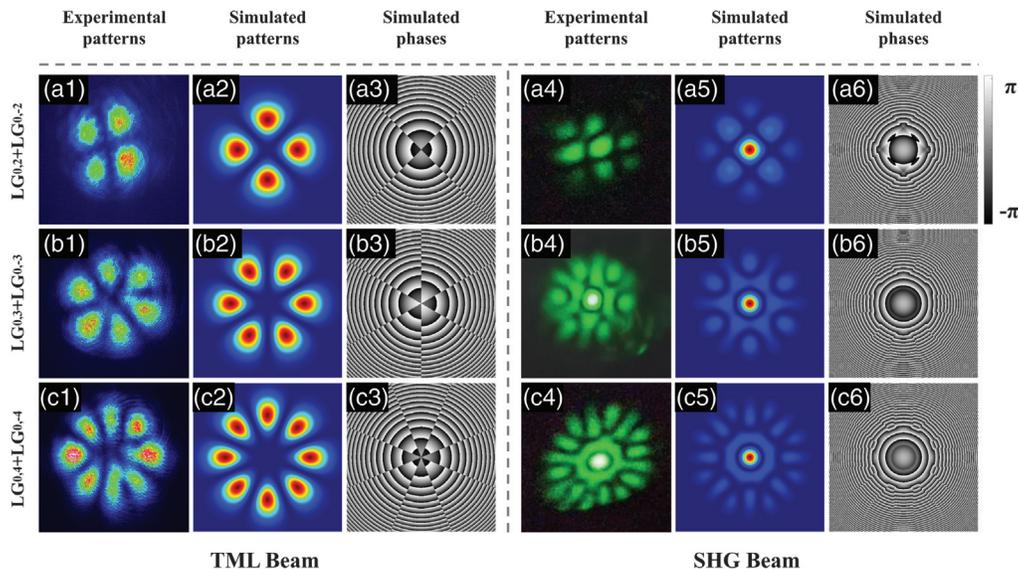
**Fig. 7** The experimental and simulated results for the SHG of TML beams that are composed of  $LG_{0,1} + LG_{0,-1}$  modes. (a)–(c) The combinations are  $LG_{0,2} + LG_{0,-2}$ ,  $LG_{0,3} + LG_{0,-3}$ , and  $LG_{0,4} + LG_{0,-4}$ , respectively. (a1)–(c1) and (a4)–(c4) Experimentally measured far-field beam patterns of TML beams and SHG beams. (a2)–(c2), (a3)–(c3) and (a5)–(c5), (a6)–(c6) are the corresponding simulated far-field patterns and phases.
