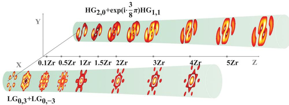
**Fig. 5** Variations of two SHG beam patterns of TML beams in the near field. The upper one is the SHG beam of the TML beam of  $HG_{2,0} + \exp(i \cdot 3\pi/8)HG_{1,1}$ , and the lower one is the SHG beam of TML beam of  $LG_{0,3} + LG_{0,-3}$ .
