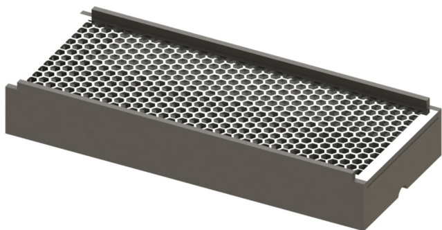
Fig. 6 Engineering drawing of a CAT grating in a holder. The L2 support structure is visible as the hexagonal structure that is 0.5-mm deep; the grating is a 4\text{-}\mu\text{m} layer on top, with the dispersion along the long axis.
