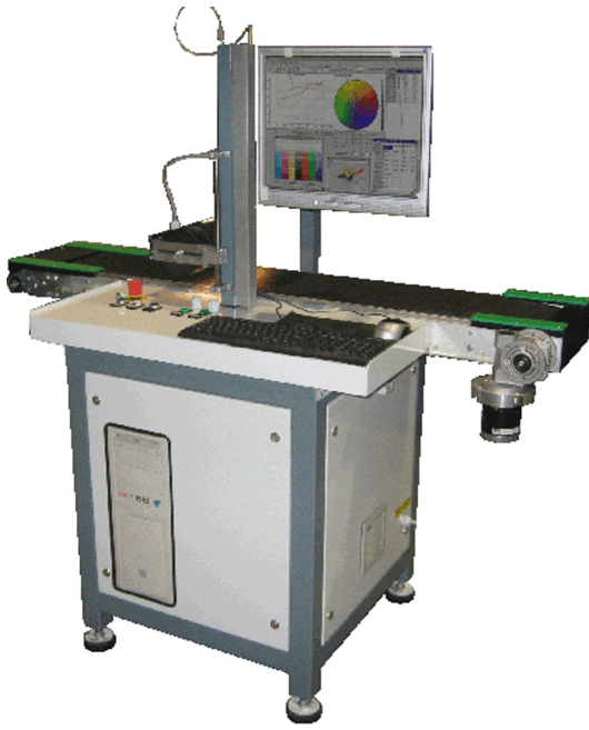
Fig. 3 HSI based architecture employed for the acquisition of the kidney stones spectra.
