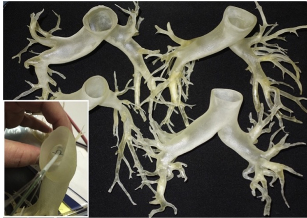
Fig. 8 An example of an ATC phantom. This phantom mimics the human pulmonary artery. This phantom was 3D printed using a PolyJet® printer. The bottom left hand of the image shows an example of a catheter being placed into the phantom.
