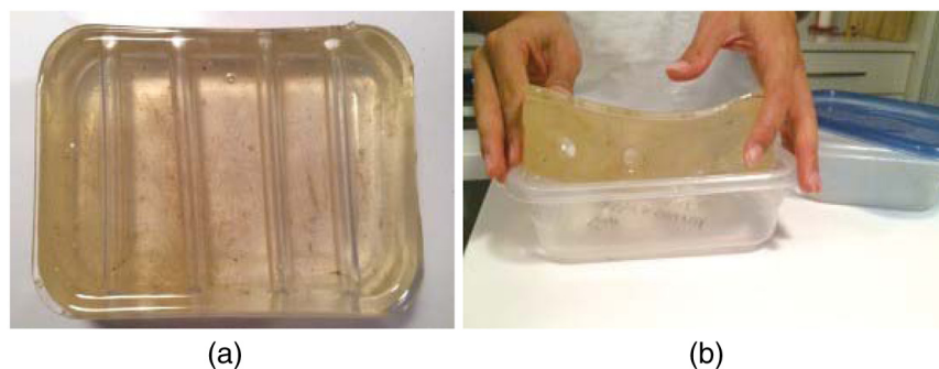
Fig. 5 An example of an embedded tube/channel phantom. PVC pipe was used to create four channels within a ballistic gel. The phantom was then sealed and used for ultrasonic measurement. (a) A top view of the phantom and (b) the channels from the side.
