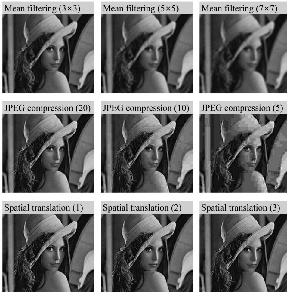
Fig. 9 Comparison of image similarity for different distortion levels (the numerics in parentheses indicate filter sizes of MF, quality factors of JPEG compression, and pixel amounts of ST).
