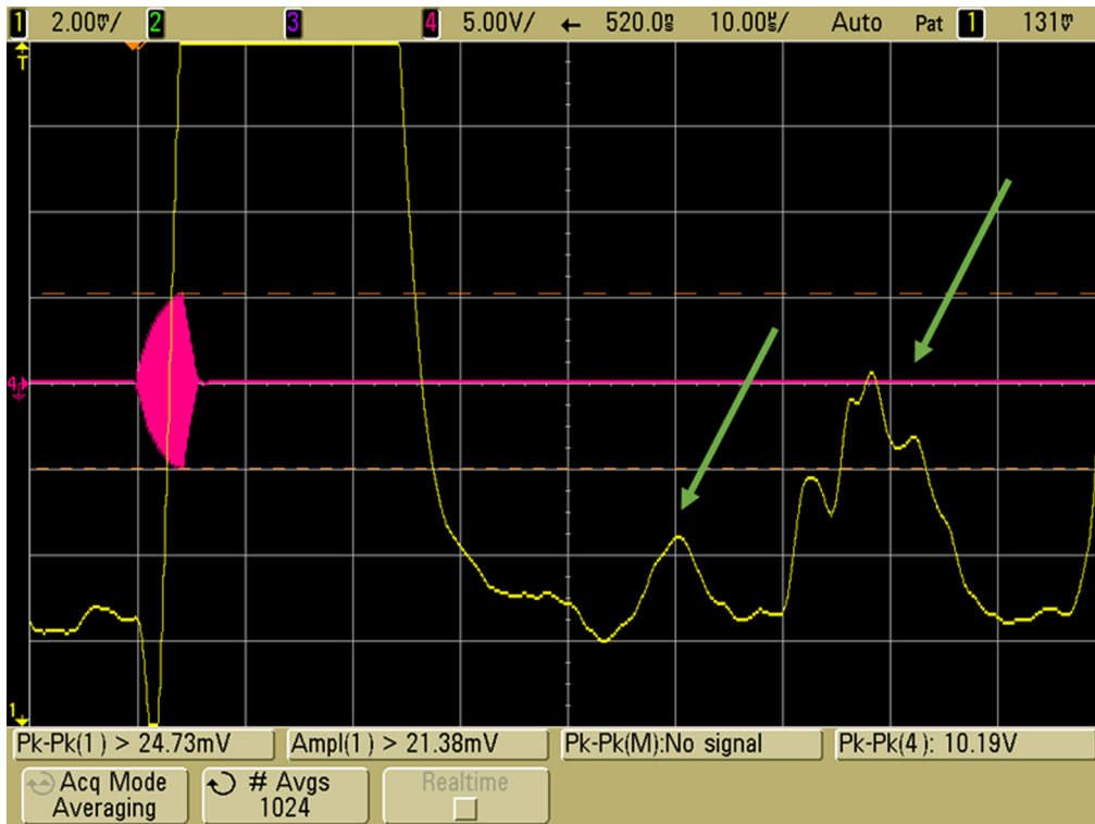
Fig. 10 EMAI signal from a section of beef liver suspended in saline. The pink tracing displays the 4- \mu s RF burst with active damping. The yellow trace is coherent processing amplitude envelope from the receiver. Green arrows indicate the position of the two macroscopically distinguishable sections of liver including vessel stubs.
