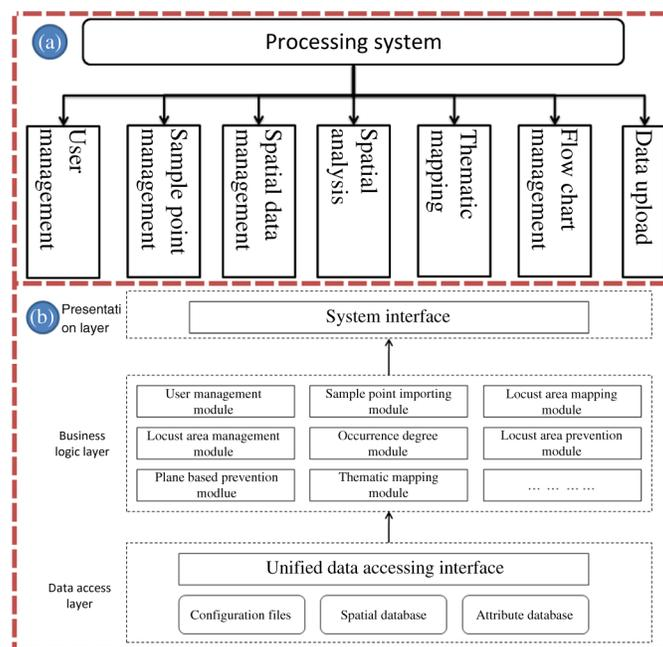
**Fig. 5** Processing system design diagram. (a) Processing system function diagram. (b) Software architecture diagram of processing system.
