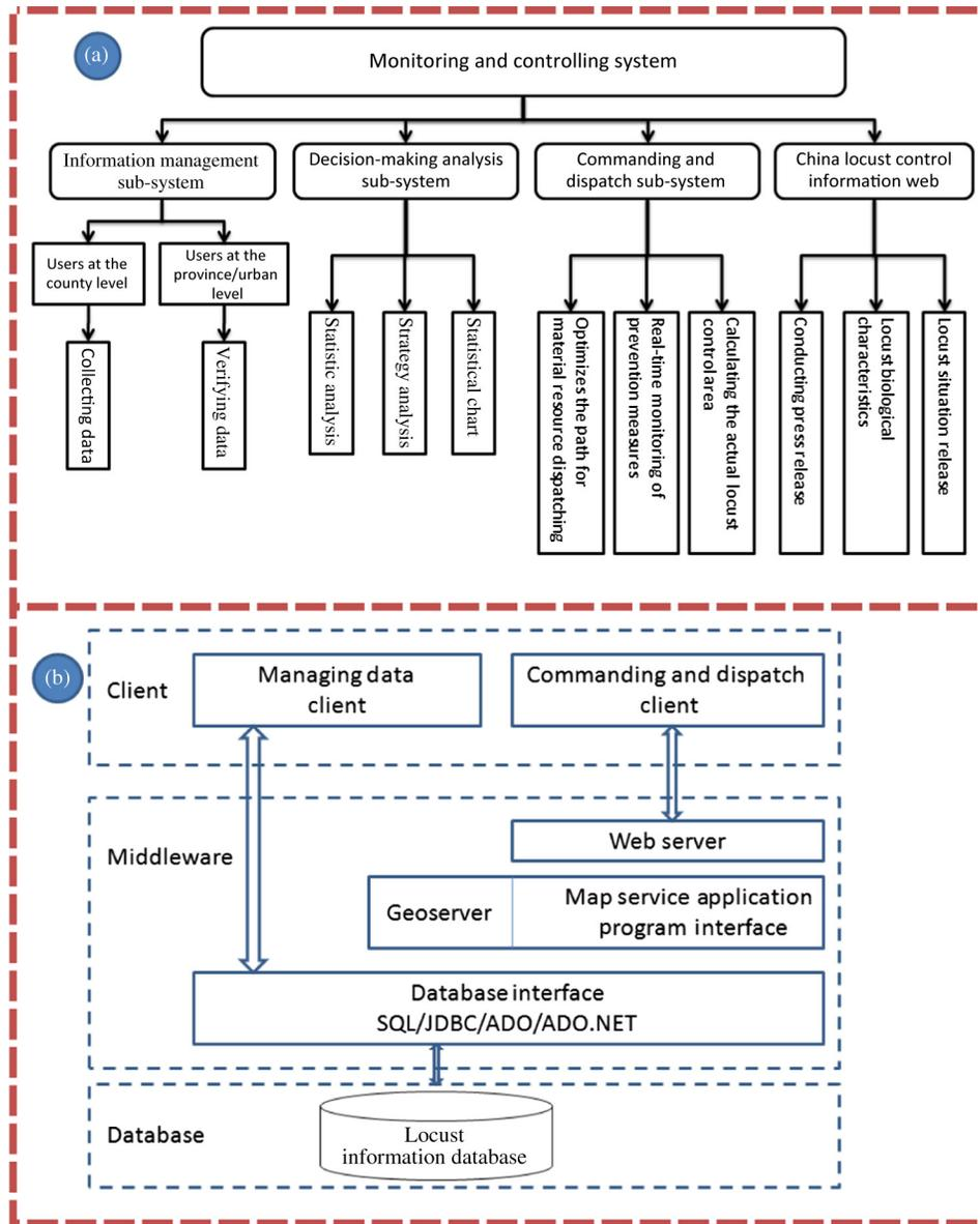
**Fig. 7** Monitoring and controlling system design diagram. (a) Monitoring and controlling system function diagram. (b) Software architecture diagram of monitoring and controlling system.
