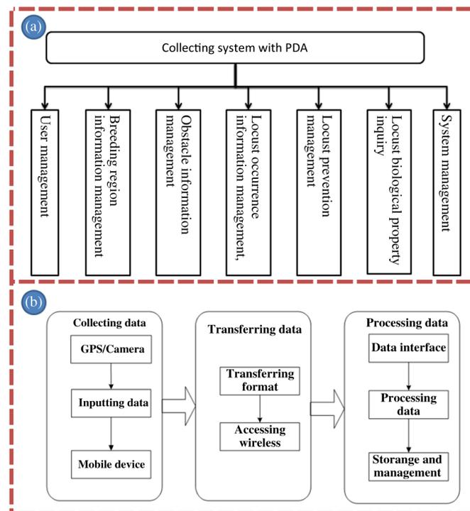
**Fig. 4** Collecting system with personal digital assistant (PDA) design diagram. (a) Collecting system with PDA function diagram. (b) Working flowchart of collecting system with PDA.
