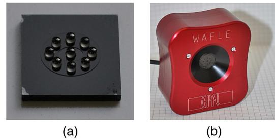
**Fig. 5** (a) Image of the back-side of the fabricated objective. It has a square shape with a side length of 11 mm. (b) The finished device. The objective is glued onto the black support and aligned in front of the camera sensor. The dimensions of the case are  $6.0 \times 5.5 \times 3$  cm<sup>3</sup>.
