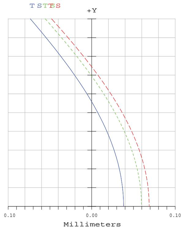
**Fig. 3** Plot of the field curvature for the designed lens (diameter of the aperture stop of  $0.33 \text{ mm}$ ) for field angles up to  $40 \text{ deg}$  and for the wavelength of  $486 \text{ nm}$  (blue, continuous),  $589 \text{ nm}$  (green, short dash), and  $656 \text{ nm}$  (red, long dash).
