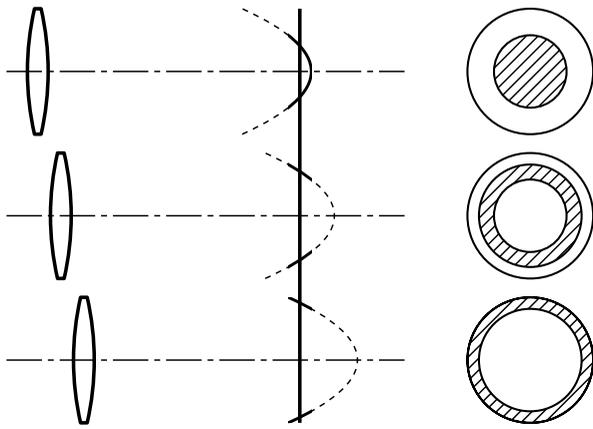
**Fig. 1** Drawing of three-lens systems forming three images on a flat sensor represented by a vertical continuous line (center). The three lenses are identical. They form sharp images over a curved field (dashed line). Each lens is located at a different axial position and its curved field crosses the sensor at a different height. On the right, the three fields are represented. The hatched areas indicate the field areas sharply imaged on the sensor.
