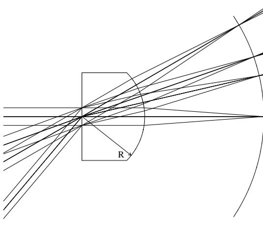
**Fig. 2** Schematic drawing of the thick plano-convex lens with the aperture stop at the plane surface, a design close to the rear landscape lens,<sup>22</sup> but with a single curved surface. The arrow indicates that the centre of curvature of the convex surface is at the centre of the aperture.
