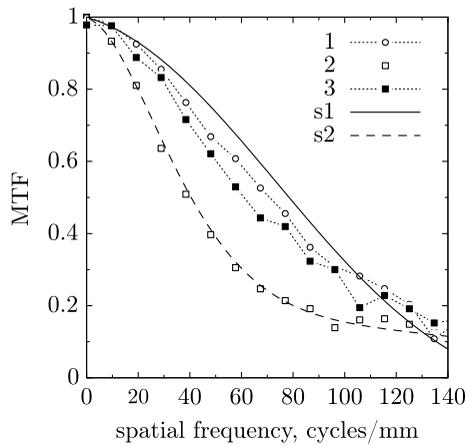
**Fig. 7** Measured MTF plot for the three image locations shown in Fig. 6. The location (1) is in the center and (2) at a field angle of 33 deg of the central channel image. The location (3) is in the satellite image corresponding to the location (2). The continuous (S1) and dashed (S2) lines represent the simulated MTF for the positions (1) and (2), respectively.
