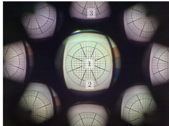
**Fig. 6** Raw image of a grid acquired with the multichannel objective. The central circle extends to a field angle of 27 deg and the external one to 40 deg. The central image is sharp up to about 27 deg. The satellite images are sharp between 27 and 40 deg as designed. The numbers 1 to 3 indicate the location of the modulation transfer function (MTF) measurements shown in Fig. 7.
