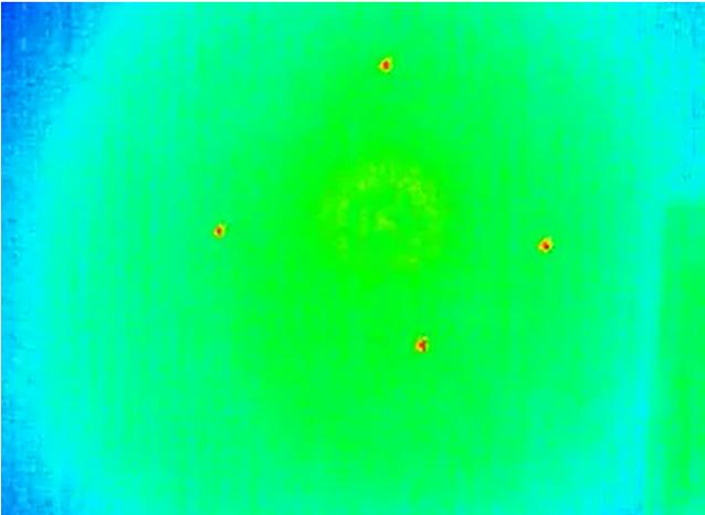
**Fig. 11** Video recording of multiple beams steered simultaneously across the field of engagement. A delay of 300 ms is inserted between each movement to ensure that the free-running camera captures every movement. (Video 4, mp4, 1.0 MB [URL: <https://doi.org/10.1117/1.OE.57.2.027108.4>].)
