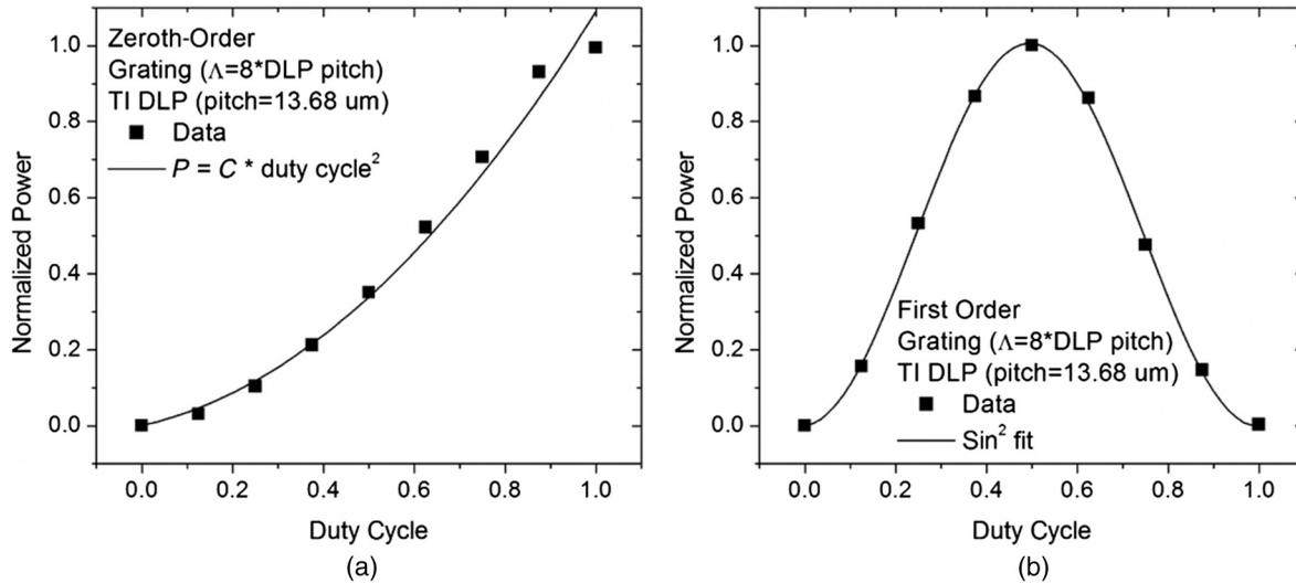
**Fig. 2** (a) Normalized power in the zeroth-order as a function of spatial duty cycle of an 8 pixel period grating and (b) the normalized power in the first order as a function of spatial duty cycle. The lines drawn through the data are curve fits to the data.
