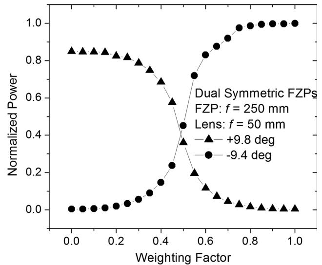
**Fig. 9** Normalized power in each beam for a dual symmetric composite FZP as a function of the relative weighting factor. As the relative weighting factor is varied, the power is transferred from one beam to the other. See Video 3. The power asymmetry is due to alignment. This asymmetry is also seen in Figs. 3 and 4 and its origin is discussed above.
