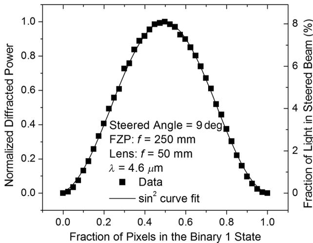
**Fig. 7** Normalized power diffracted into a beam steered at 9 deg as a function of the percent of pixels in the binary 1 state. The line through the data is a  $\sin^2$  curve fit to the data. Intensity control is demonstrated in Fig. 8.
