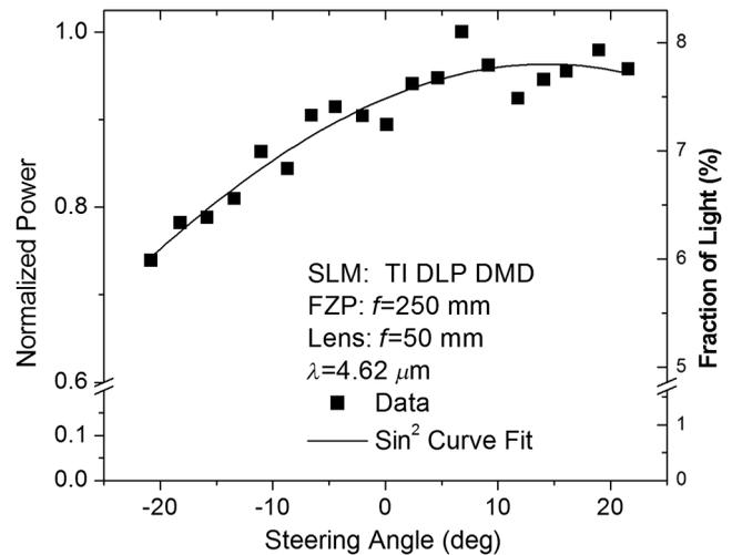
**Fig. 4** Normalized power in the recollimated steered beam as a function of steering angle. The maximum angle is limited by the field-of-view of the recollimating lens. Beam steering is demonstrated in Fig. 5.
