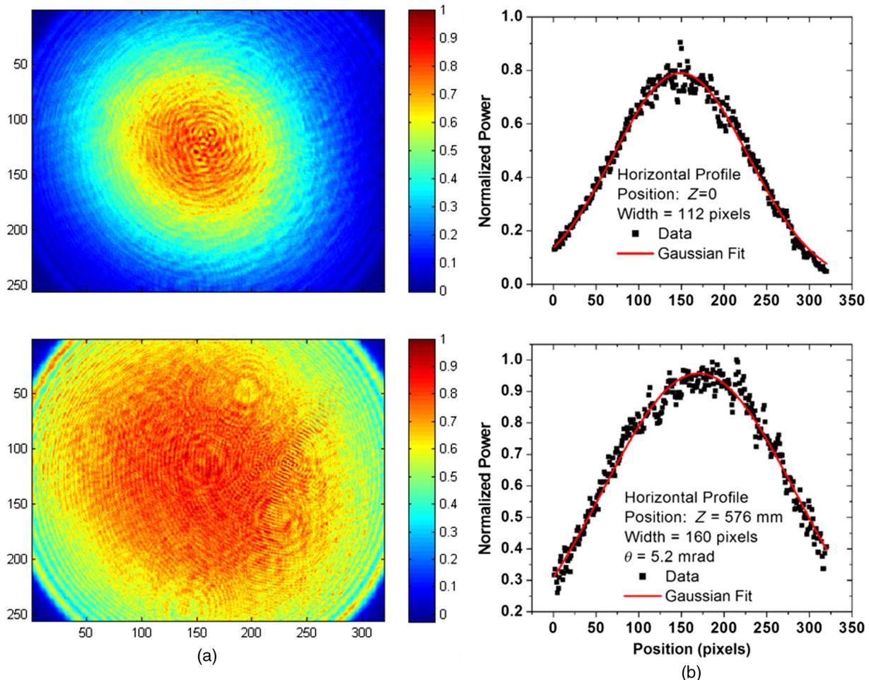
**Fig. 6** Profile of the steered laser beam measured at two positions along the propagation of the beam. (a) Images of the laser beam at the two positions and (b) the corresponding line profile of the laser beam. The distance between the two positions is 576 mm. The line drawn through the data points is a Gaussian curve fit. The measured divergence is 5.2 mrad.
