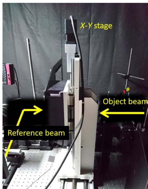
**Fig. 2** Experimental setup of holographic wavefront printer.
