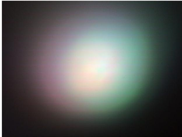
Figure 6. Color mixing result with the Ledil lens. Mixing is improved, but not good.
