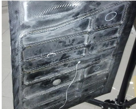
Figure 12. CFRP panel with stiffeners (example of real aerospace structure).
