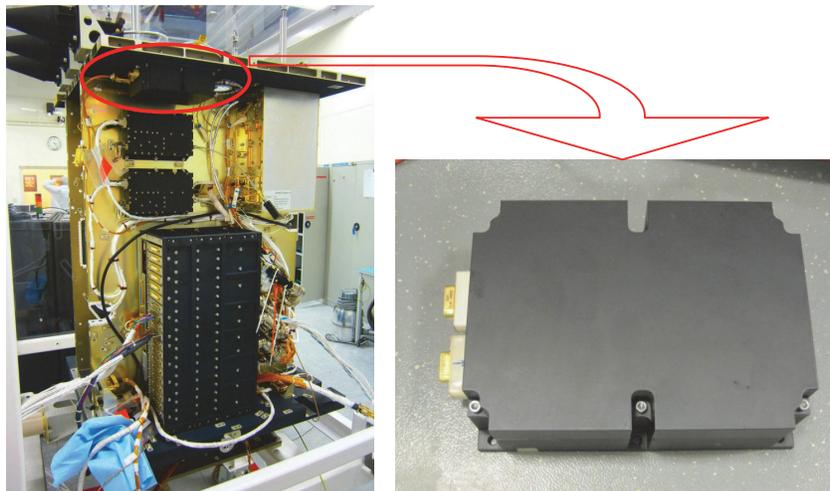
Figure 8: HERMOD PFM payload before(right) and after (left) integration on Proba-V platform.
