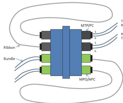
Figure 4 Design of the HERMOD optical assembly including the 4 channels.
