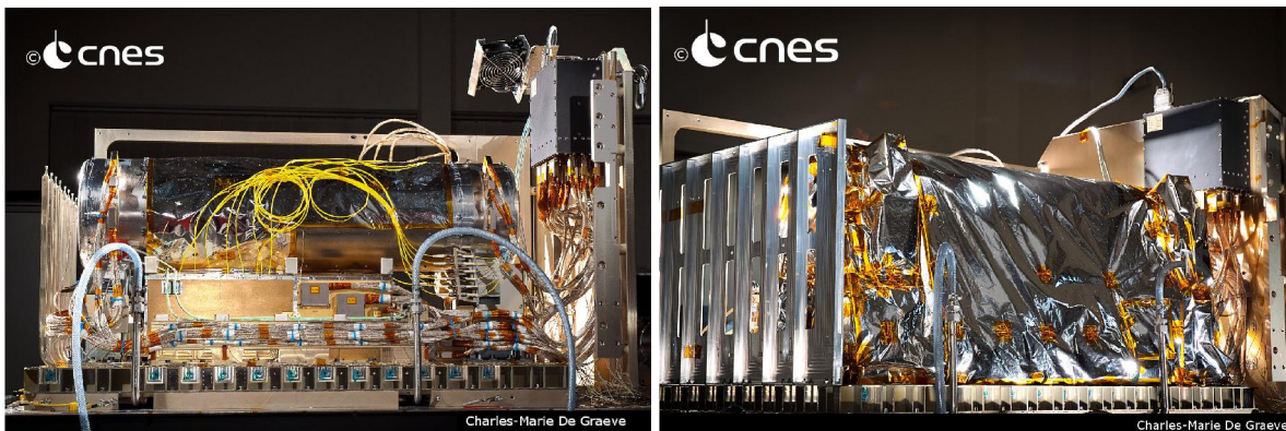
Fig. 1. PHARAO flight model before and after integration of the MLI protection.
