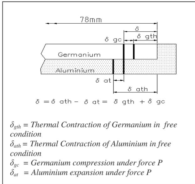
Fig. 3 Behaviour under bimetallic force
