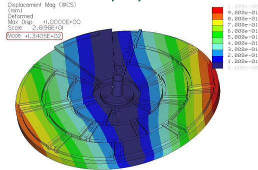
Fig. 10 Eigen value analysis of the wheel
