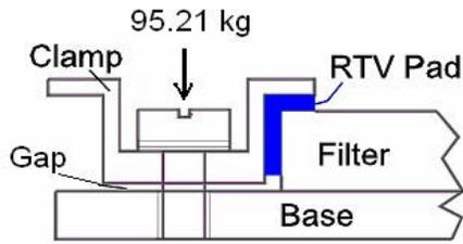
Fig.6 Soft Mount Assembly with gap
