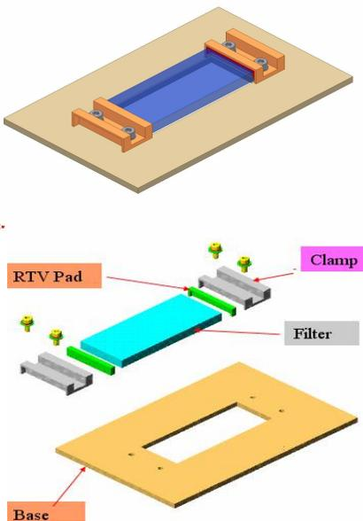
Fig.5 Assembly and Exploded Views of Soft Mount
