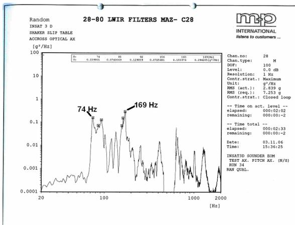
Fig. 13 Wheel modes in dynamic tests
