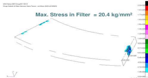
Fig. 8 FEA thermal stress results for Filter while in flexure mount
