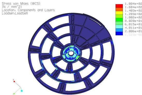
Fig. 11 Thermal stress on the wheel
