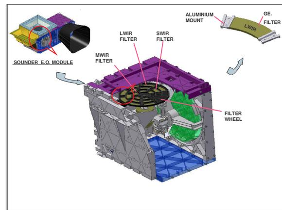
Fig.1 Filter Wheel Configuration and Filter Mount
