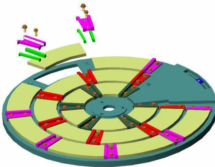
Fig.2. Filter wheel assembly
