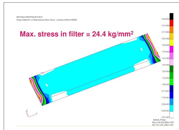
Fig. 4 FEA results of bimetallic stress on the Filter
