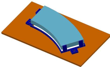
Fig. 7 Flexure Mount
