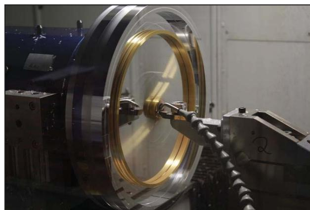
Fig. 5: Single Point Diamond Turning of M2
