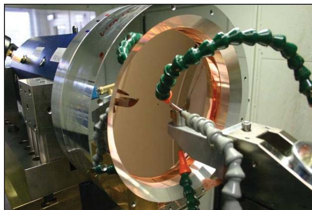
Fig. 4: Single Point Diamond Turning of M1
