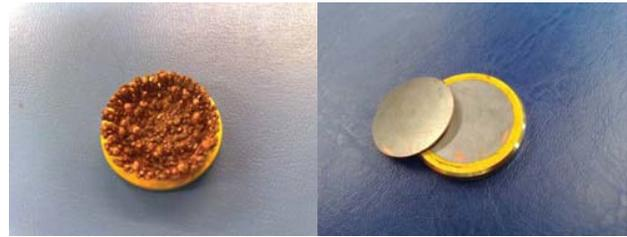
Fig. 7: Problems during coating development (left: unexpected Cu growth, right: poor adhesion)
