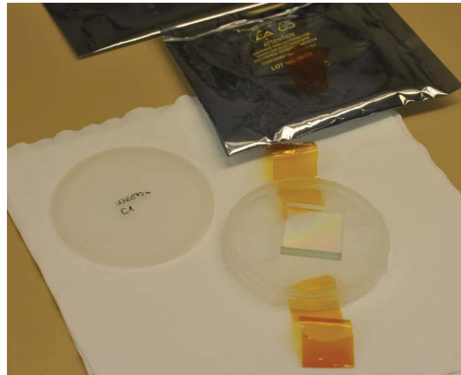
Figure 4 IOF lithographic grating
