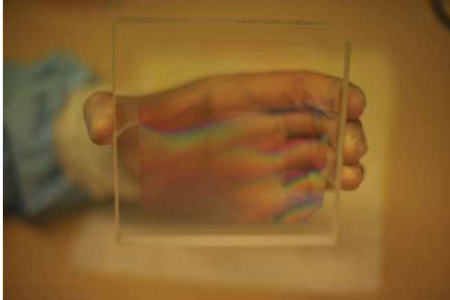
Figure 13 CSL Volume Bragg grating
