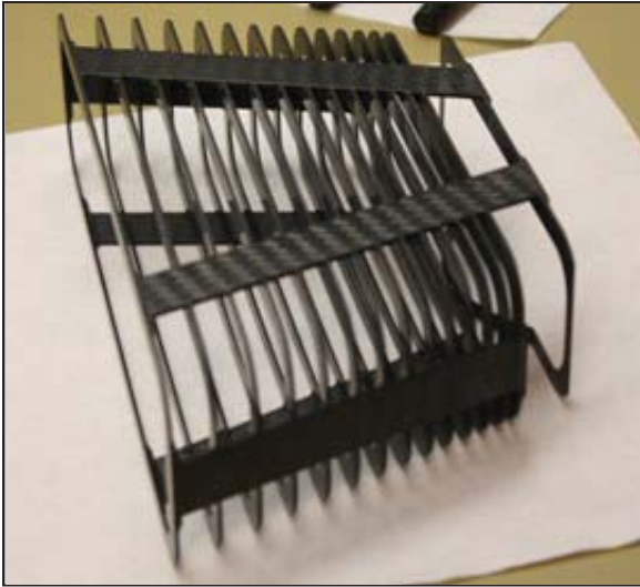
Fig. 7. Protector buffer in Carbon Fibre Reinforced Plastic.
