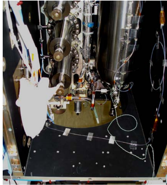
Fig.12: P/T and HT sensors mounting on Proba2.
