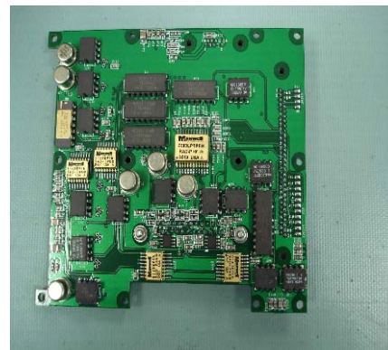
Fig. 3: Photograph of the low-power flight DAQ (Data Acquisition) PCB.
