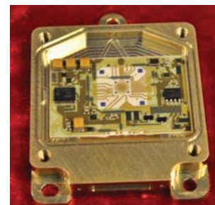
Figure 7: Ceramic chip carrier carrying the SMD peripheral electronics.
