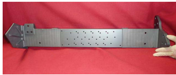
Fig. 9. The VNIR detector support (3.6 kg)
