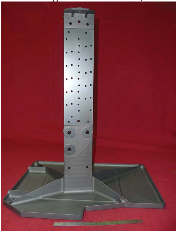
Fig. 8. The SWIR detector support (5.4 kg)
