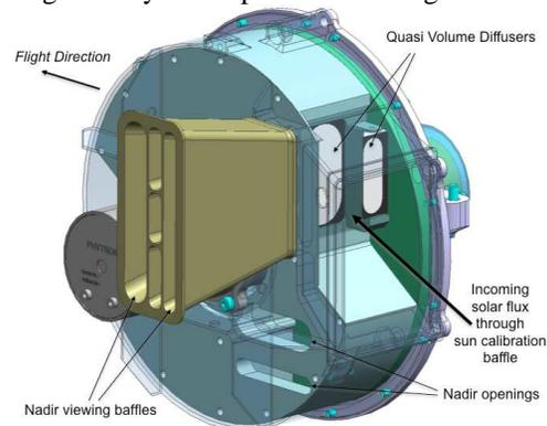
Fig. II-4 VNS Calibration mechanism
