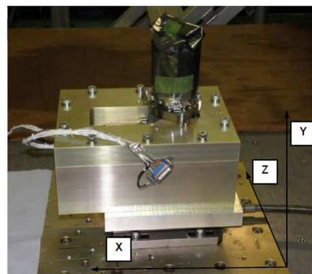
Fig. III-5 TIR CMA ECM microvibration test
