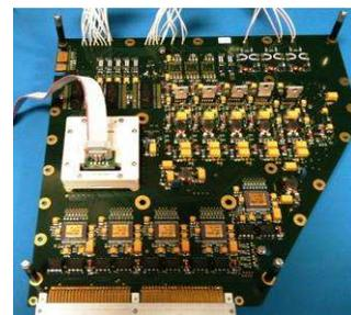
Fig. IV-1 FEE breadboard - FPGA being programmed
