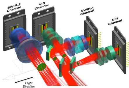
Fig. II-2: VNS camera optical configuration
