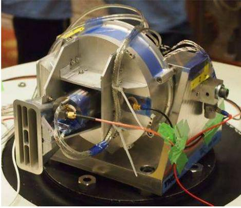
Fig. II-5: VNS life test model during vibration test at CSL
