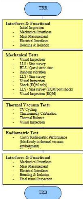
Fig. III-7 TIR CMA qualification testing campaign
