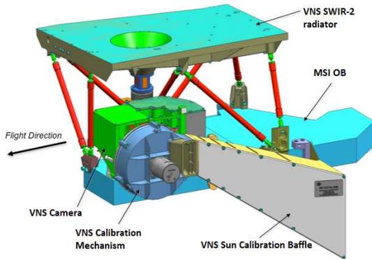
Fig. II-1 3D CAD model of the VNS
