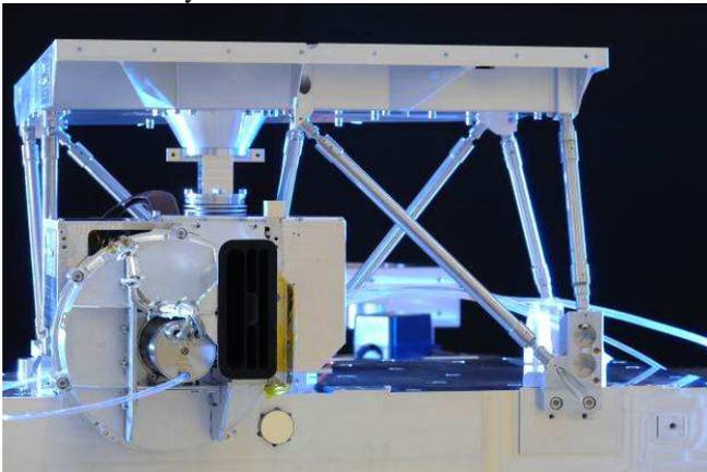
Fig. II-6 VNS ECM (Sun Baffle not assembled)
