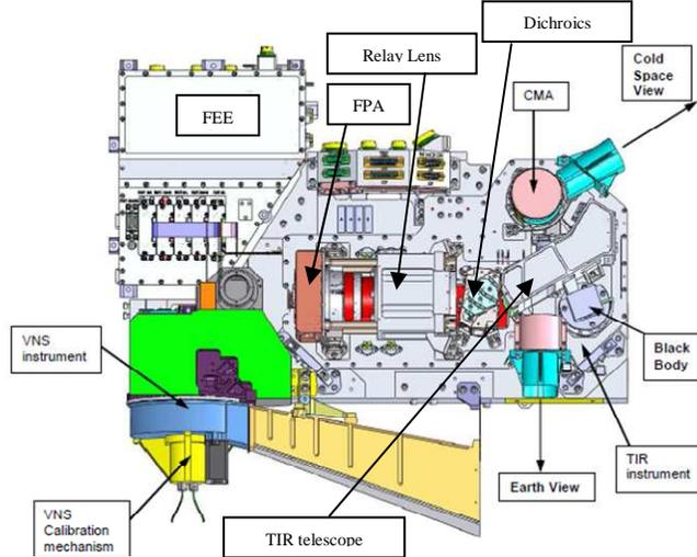
Fig. III-2 MSI OBM from above: TIR cover, SWIR2 radiator, harnesses omitted
