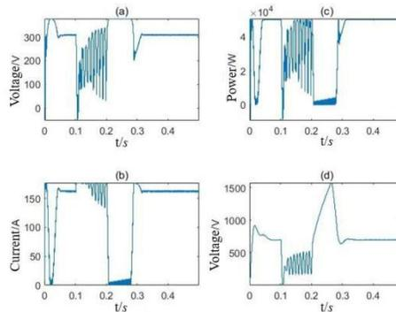
Figure 7. The output voltage, current and power of PV plant and the voltage of DC-side capacitance.
