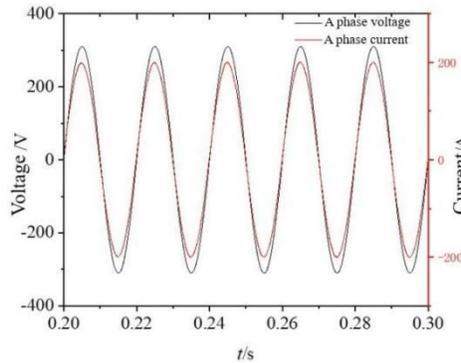
Figure 3. Voltage and current waveforms of PV A phase.
