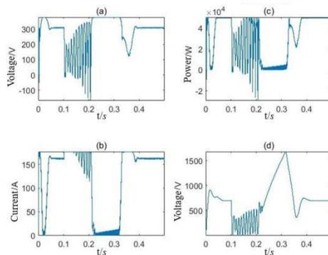
Figure 10. The output voltage, current and power of PV plant and the voltage of DC-side capacitance.
