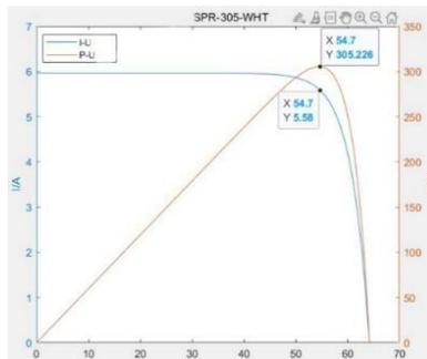
Figure 1. Output characteristic under standard working conditions.
