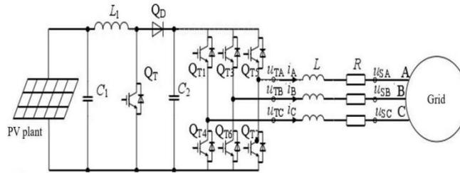
Figure 2. Structure of two-stage PV grid-connected power generation system.
