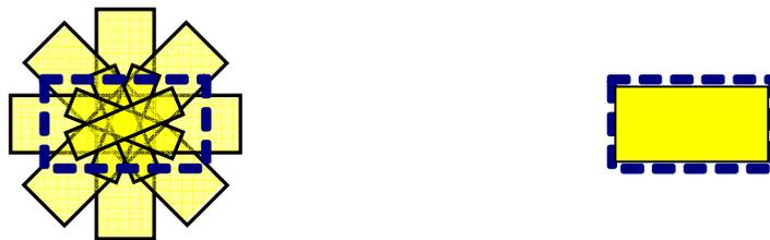
Fig. 3. The XX 3D condenser, in contrast to conventional condensers (left), can be designed to avoid the rotation of projected arc images so that it can fit rectangular apertures.
