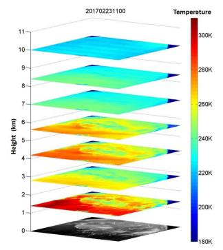
Figure 3. The 3 dimensional temperature profile obtained by geostationary interfering infrared sounder on FY-4
