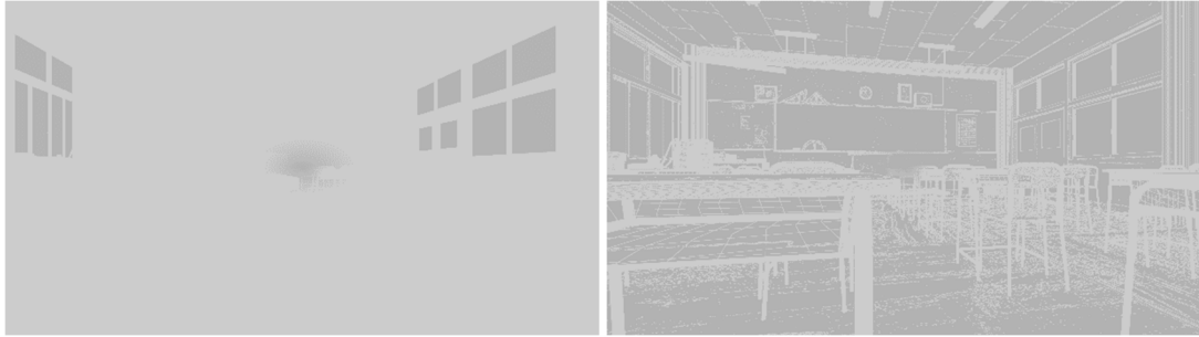
(a) (b) Figure 4. (a) TAA's blur mask. (b) ETAA's blur mask.
