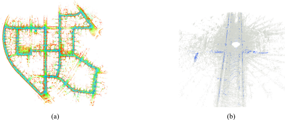
Figure 1. A KITTI dataset example using the suggested strategy. (a) shows the mapping result of the proposed method on KITTI dataset sequence 00. (b) shows a loop closure detection example, where the colorful portion represents the point cloud in the current frame and the gray portion represents the historical map.
