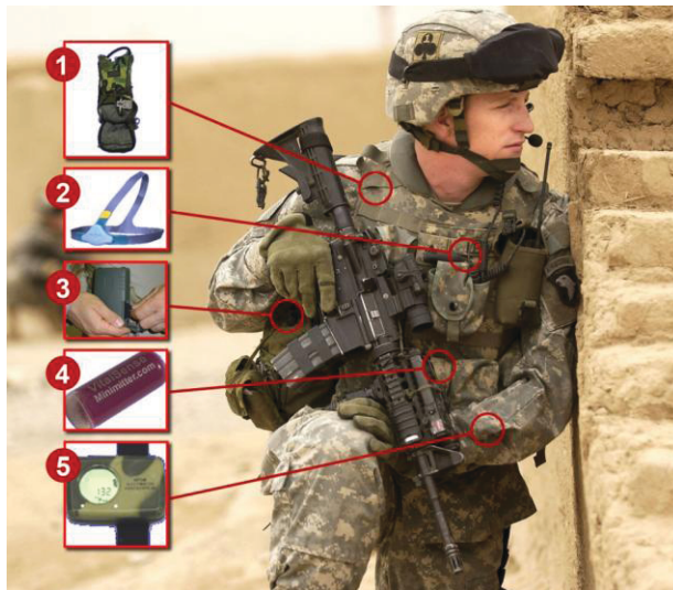
Figure 3a. The Warfighter Physiological Status Monitoring Initial Capacity system components: (1) Fluid Intake Monitor, (2) Vital Sign Detection System, (3) CPU, (4) Thermometer Pill for measuring core body temperature (Tcore), (5) Activity/actigraphy watch.
