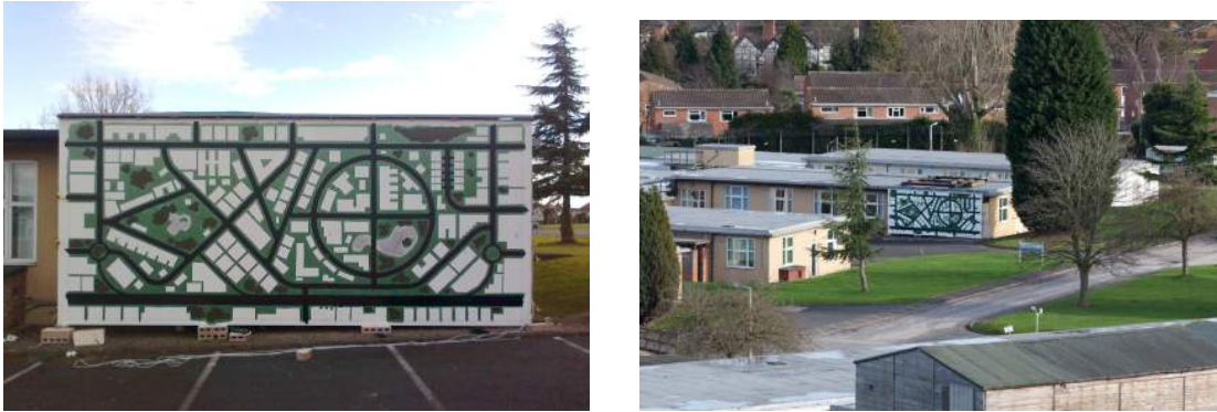
Figure 13 – Pictures of the laser tracker board left - close up, right - as seen from the laboratory
