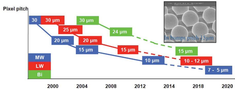
Fig. 24 Progress (solid line) and projections (dashed line) for reducing pixel size for MWIR (blue), LWIR (red), and dual-band FPA applications.
