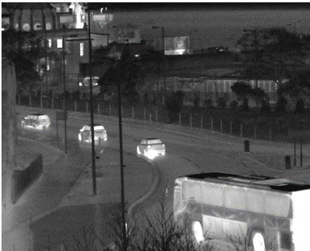
Fig. 27 Image taken at 160 K with a HgCdTe-on-GaAs FPA with 16  $\mu\text{m}$  pixels.
