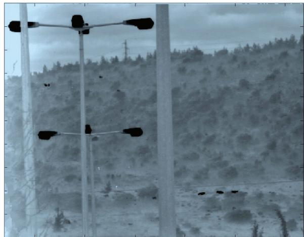
Fig. 17 Image taken at 150 K with an nBn 640 x 512 array showing an NEAT of 20 mK. The dark spots on the hill are cows.
