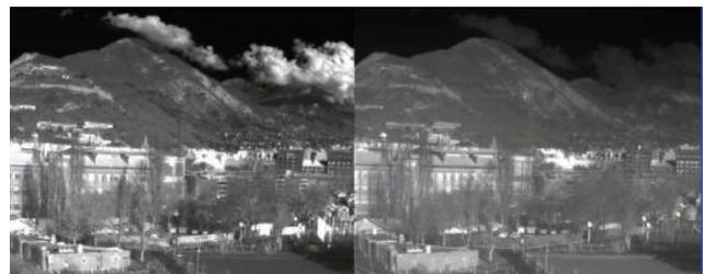
Fig. 25 Imagery taken with a dual-band MW/MW array of HgCdTe on CdZnTe having 24  $\mu\text{m}$  pitch in a 640 x 512 format.
