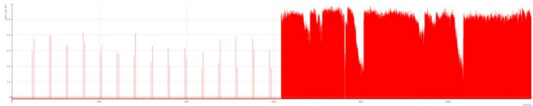
Fig. 16. On the left hand side, the EDRS-A LCT optical beam received at the OGS during the large spiraling of the EDRS-A LCT (Coarse Spatial Acquisition). On the right hand side, the EDRS-A LCT optical beam received at the OGS during the fine spiraling of the EDRS-A LCT (Fine Spatial Acquisition). Measured data from Link #2016-EDRSA-06.
