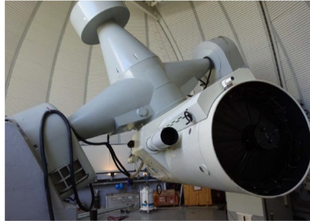
Fig. 9. The telescopes of the ESA's Optical Ground Station (OGS) used for the in-orbit test of the EDRS-A LCT. The Transmitter Telescope (guide telescope on the center of the image) is mechanically attached to the Receiver Telescope (large aperture to the right), a 1-meter Ritchey-Chrétien/Coudé telescope supported by an English mount.
