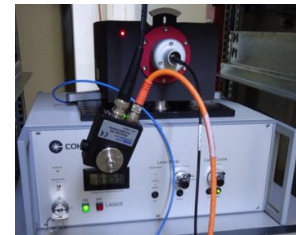
Fig. 11. The Mephisto diode pumped monolithic Nd:YAG Seed Laser from Coherent.
