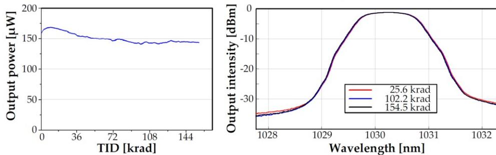
Fig. 9: Left: Optical output power of the SESAM based Yb-fiber laser during gamma radiation test. Right: Optical output spectrum at different TID levels.
