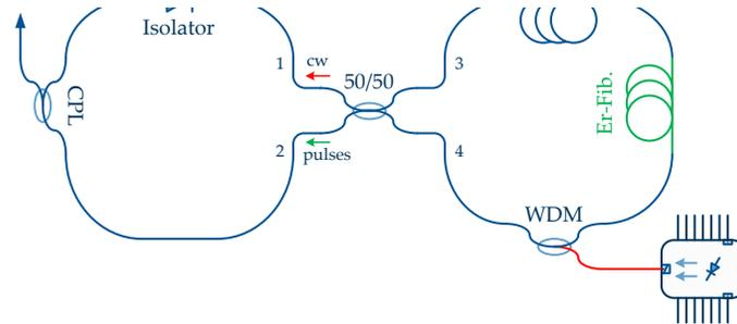
Fig. 5: Nonlinear Amplifying Loop Mirror (NALM) based oscillator from [17].
