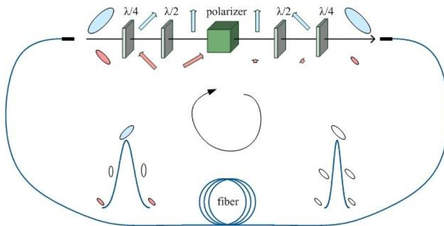
**Fig. 3: Basic principle of the nonlinear polarization rotation mode-locking. The high intense pulse center (light blue) is rotates in the fiber more than the low intense pulse wings (light red). The low intense pulse wings with a certain polarization are filtered out by waveplates and a polarizing element.**
