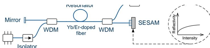
Fig. 4: Schematic illustration of a SAM based laser oscillator. The SAM acts as mode-locking element in that sense that only high intense light is reflected back.
