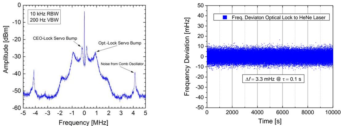
**Fig. 11:** Beat signal when the SAM based comb is stabilized to a HeNe laser (left) and corresponding frequency stability of optical lock (right) [20].
