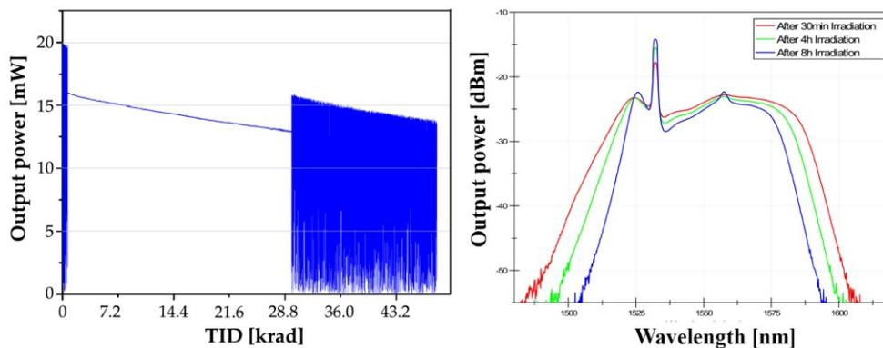
Fig. 8: Left: Optical output power of the NLPR Er-fiber laser during gamma radiation test. Right: Optical output spectrum showing a large cw-peak which increases with total dose.
