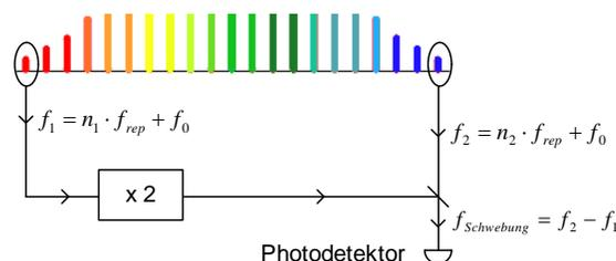
Fig. 6: Basic idea to detect the CEO frequency. The longer wavelength part (~2µ) is frequency doubled in a SHG crystal and then superimposed with the fundamental light (1µ).
