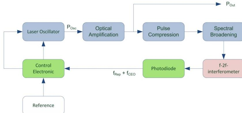
Fig. 2: Block diagram of a fully stabilized optical frequency comb.
