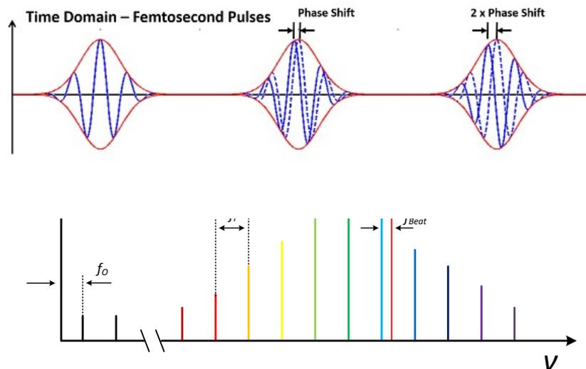
Fig. 1: Top: Pulse train in time domain illustrating the envelope (red) of the electrical field (blue). Bottom: Illustration of the different frequencies obtained by Fourier transformation of the pulse train in time domain.
