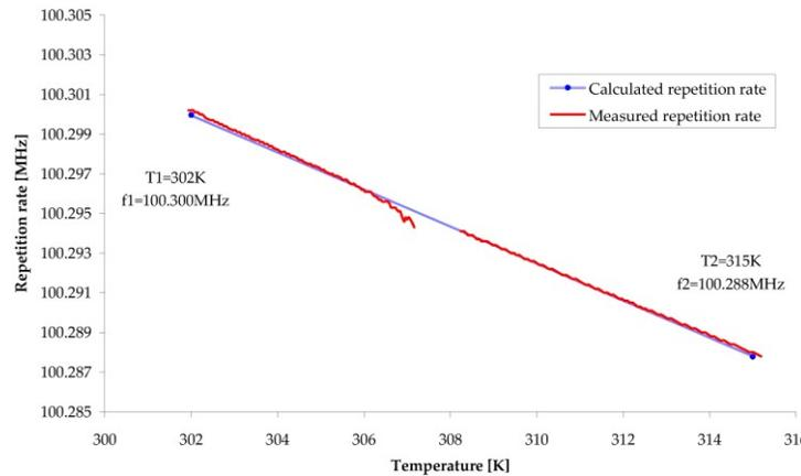
Fig. 7: Measured repetition rate ( $f_R$ ) as function of temperature (red) and theoretical calculated curve.
