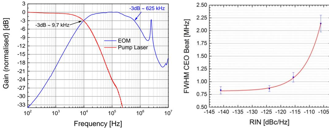
**Fig. 10:** Left: Transfer function measurements for the stabilization actuators (pump diode and integrated EOM) [18]. Right: CEO linewidth (FWHM) as function of the relative intensity noise (RIN) of the pump diode.
