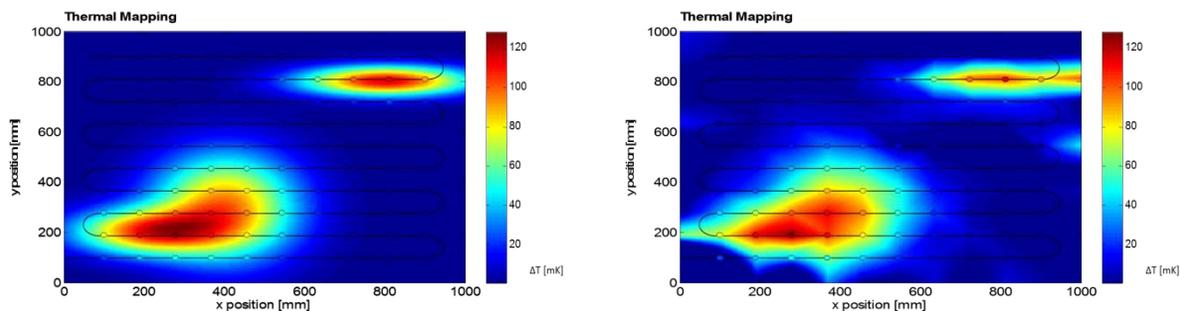
Figure 8: Example Thermal Mapping capability; On the left the original temperature map is displayed, on the right the reconstructed temperature map based on current measurement capabilities. The Temperature range is 120 milli-Kelvin
