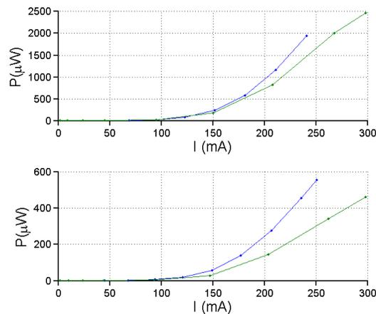
Figure 1: Current vs output power for the two packages pre and post irradiation (blue and green resp.) Top: ESTEC sample 9-40, Bottom: KVI sample 10-16.
