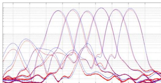
Figure 2: Indicative spectral response of 6 AWG output channels on chip 314-1-436 pre- and post-exposure (X-axis: wavelength, Y-axis: transmission (log-scale). Red and Blue resp., normalized).
