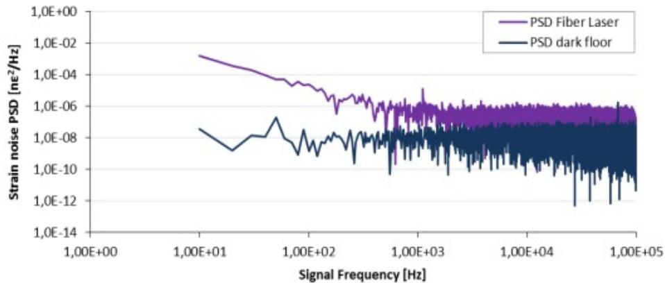
Figure 4: Power spectral density of the dark noise floor and fiber laser noise.
