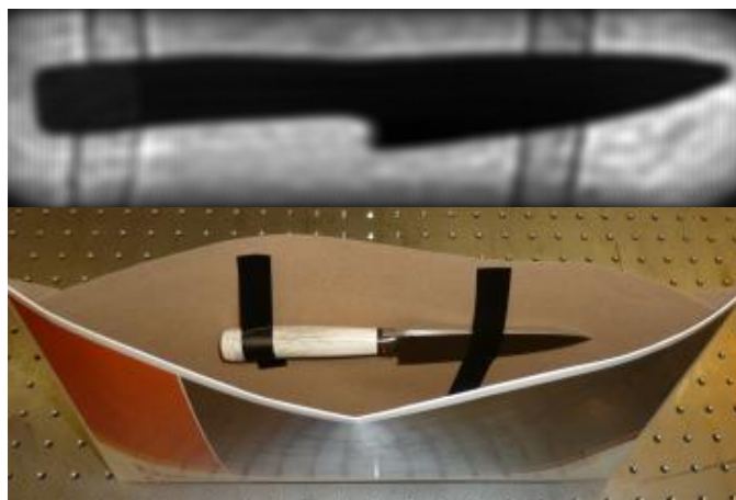
Fig. 4. THz mosaiced image taken at 432 \mu\text{m} of a knife seen through a cardboard mailing envelope (top) and visible images showing the knife hidden inside the envelope (bottom).
