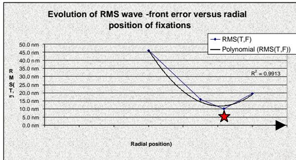
**Fig. 4 Optimisation of radial position of fixation**
