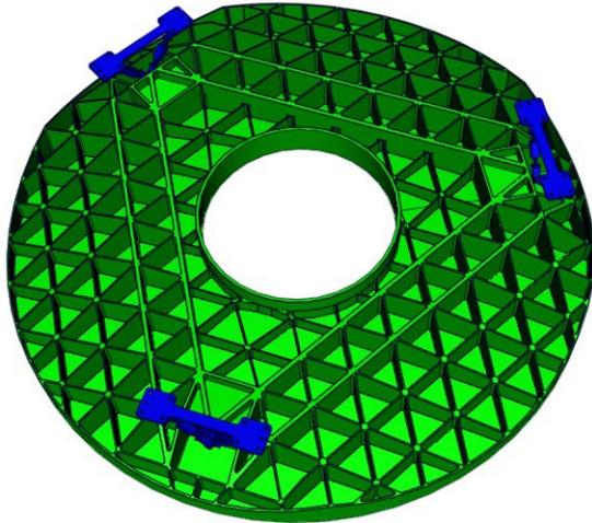
Fig. 13 Optimized SNAP mirror design
