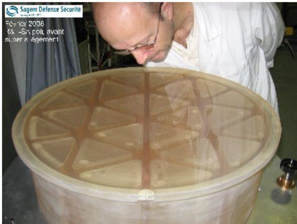
**Fig. 9 SAGEM second breadboard after rough
