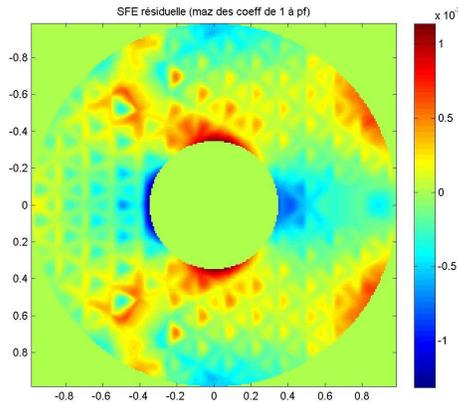
Fig. 14 Optimized SNAP mirror under gravity – interferometric view
