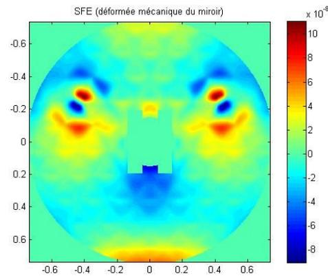
**Fig. 7 Optimized mirror under gravity – interferometric view**
