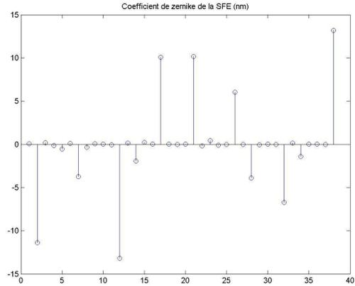
Fig. 15 Optimized SNAP mirror under gravity – ZFR Zernike decomposition
