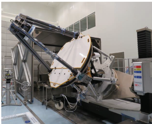
Figure 8. Active telescope at the end of the integration phase with the secondary mirror already integrated using theodolites.
