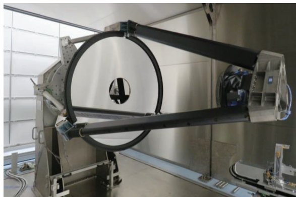
Figure 9. The “all in” alignment configuration requiring the minimum optical support equipment: an auto-collimating flat mirror (not shown) in front of the telescope equipped with its focal plane.
