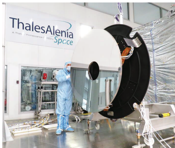
Figure 1. Fully equipped M1 Mirror (optical coating and flight Silicon Nitride isostatic mounts) during vacuum thermal cycling configuration set-up. This 1,5 m Zerodur equipped mirror has a total surfacic mass of 25 kg/m 2 .
